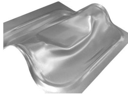
Figure 6 Actual wrinkle part while deformation
