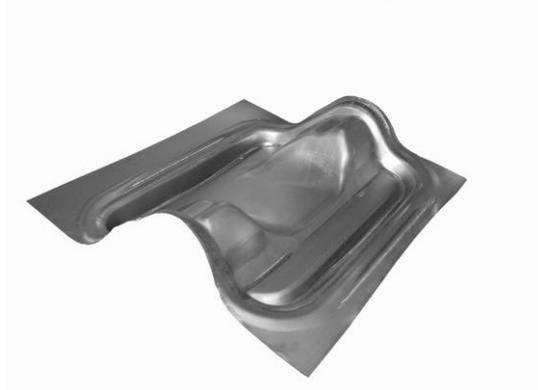
Figure 10 Experimental part with redesigned draw bead
