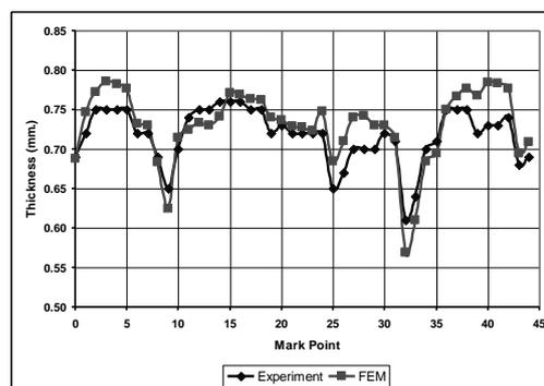
Figure 13 Thickness profile comparison of cross-section no.2
