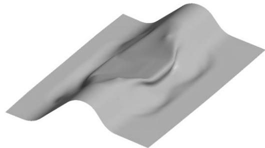
Figure 7 FEM simulation of starting wrinkle
