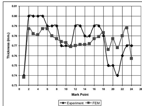
Figure 12 Thickness profile comparison of cross-section no.1
