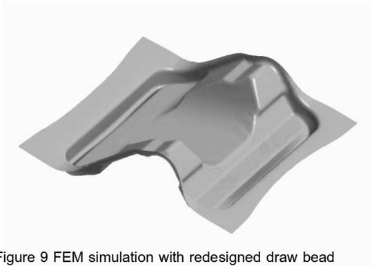
Figure 9 FEM simulation with redesigned draw bead
