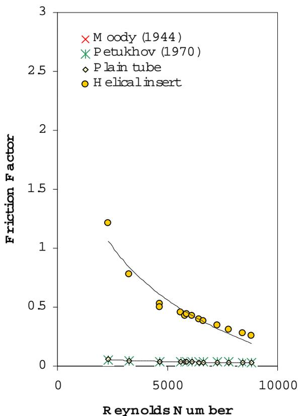
**Figure 5.** Relationship between friction factor and Reynolds number.
