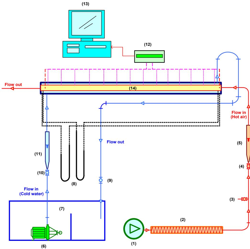
**Figure 3.** Schematic diagrams of experimental apparatus: (1) 10 hp blower, (2) an electrical heater with thermostat, (3) ball valve, (4) globe valve, (5) rotameter for hot air, (6) 1/2 hp water pump, (7)
