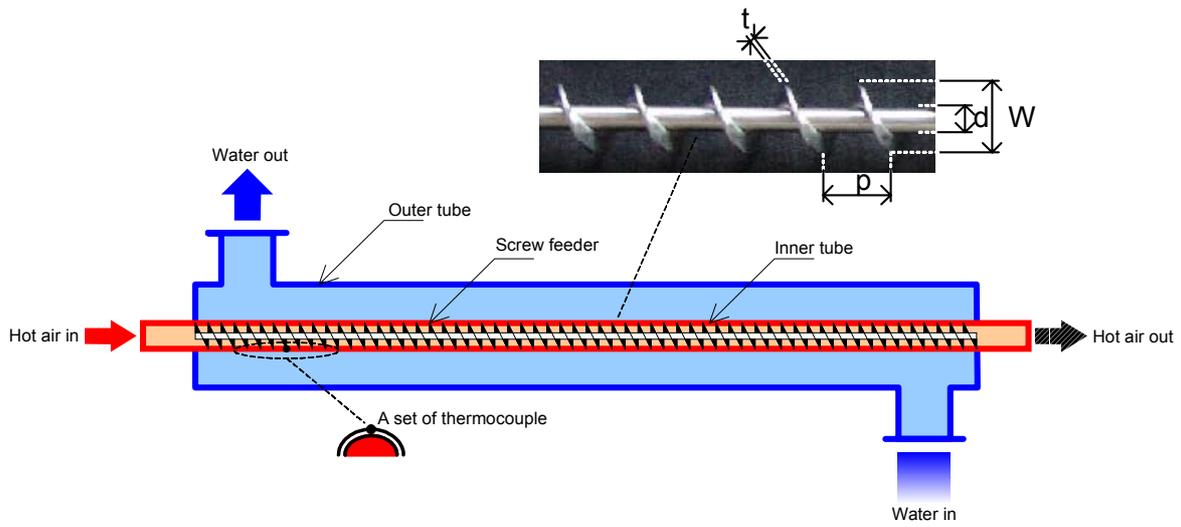
**Figure 2.** A double concentric tube heat exchanger fitted with a helical and definition of geometric parameters of the helical tape.
