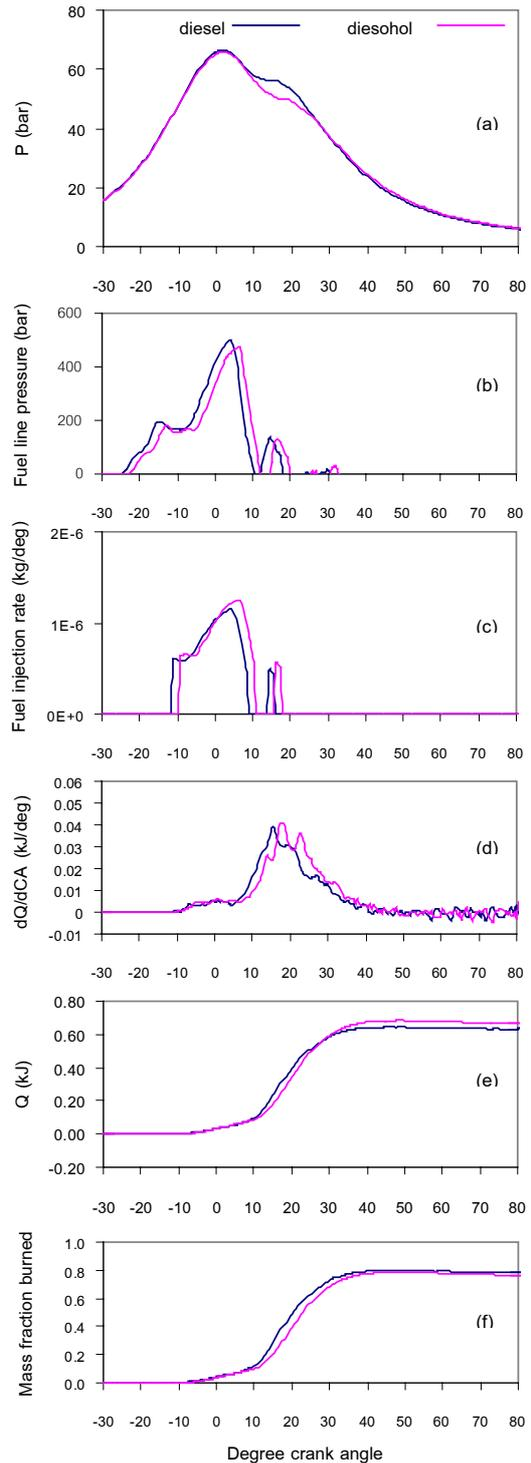
Figure 5 (a) In cylinder Pressure data, (b) Fuel line pressure, (c) Fuel injection rate (d) Heat release rate, (e) Net heat release, and (f) Mass fraction burned, at 2250 rev/min, 80 Nm.
