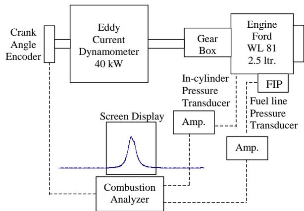
Figure 2 schematic arrangement of measuring system
