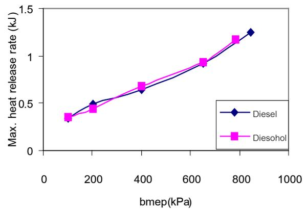
Figure 7 (b) Maximum heat release at 2250 rev/min.
