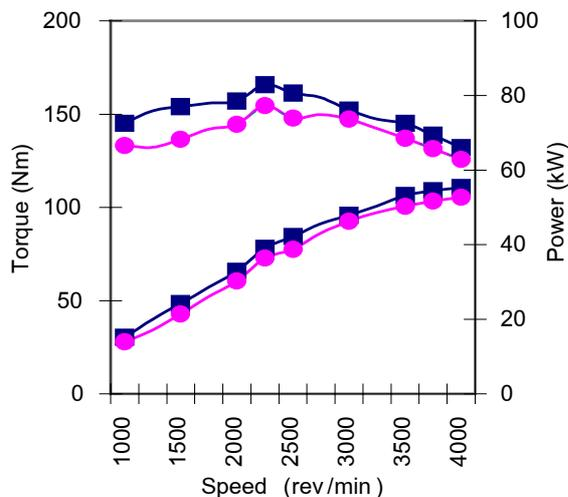
Figure 3 Maximum brake torque and power of engine.
