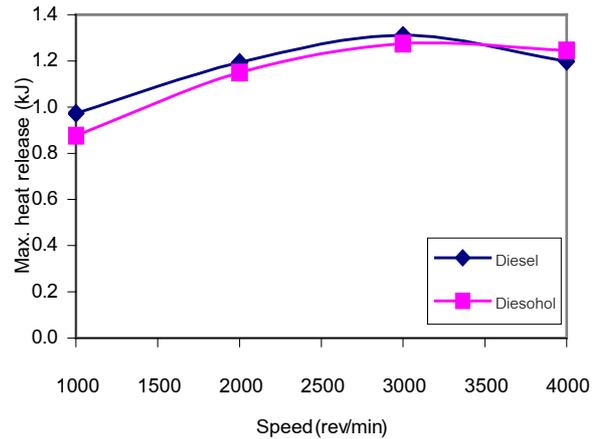
Figure 7 (a) Maximum heat release at full load.
