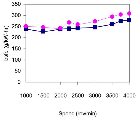
Figure 4 Brake specific fuel consumption at full load.
