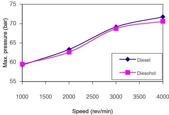
Figure 6 (a) Peak pressure at full load
