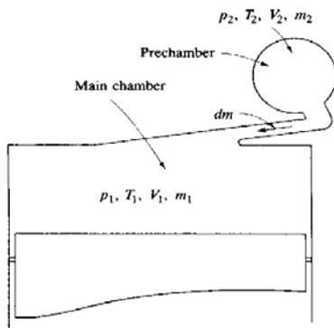
Figure 1 Schematic defining variables in main chamber (subscript 1) and prechamber (subscript 2)
