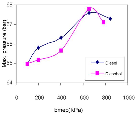
Figure 6 (b) Peak pressure at 2250 rev/min.
