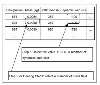
Figure 4: Identification of required parts from the search and filter mechanism
