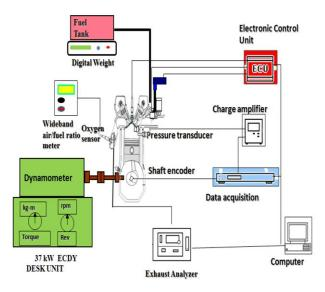
Fig. 1 Experimental set up
