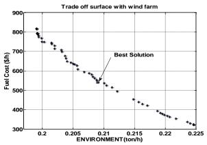
Fig.3 Best solution on tradeoff surface with wind farm in power system
