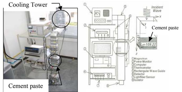
Fig. 2 The microwave experimental apparatus
