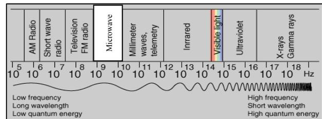
**Fig. 1** Electromagnetic spectrum
