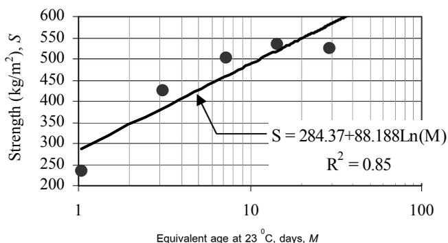
Fig. 10 A strength-maturity relationship of the 0.4-w/c cement paste
