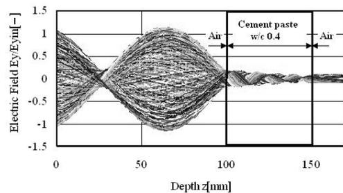
Fig. 6 A typical electric field distribution rectangular wave guide is filled with cement paste sample ( $t = 60$  sec., Power = 1000 W).
