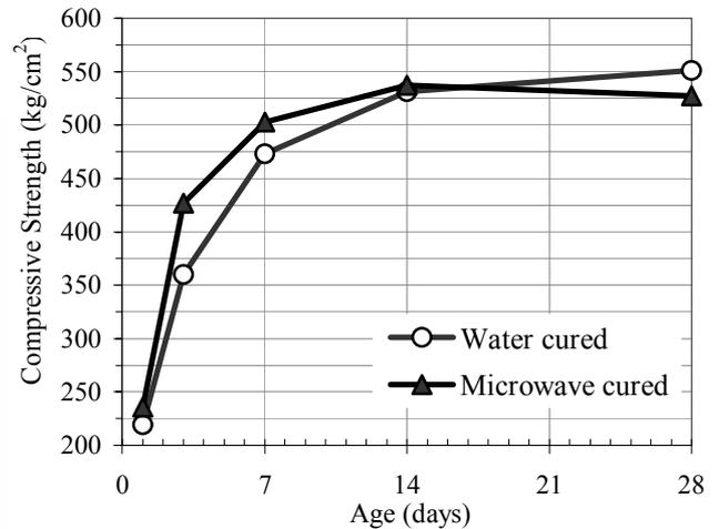
Fig. 9 Comparison of compressive strength development for different curing methods
