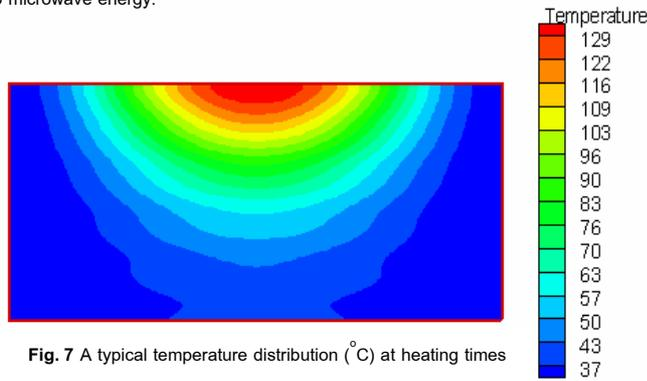
Fig. 7 A typical temperature distribution ( $^{\circ}\text{C}$ ) at heating times for 60 sec.
