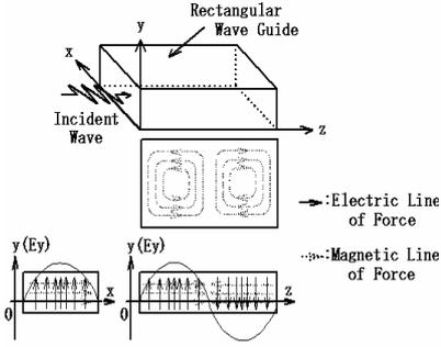
**Fig. 4** The electromagnetic field distribution on x-z plane
