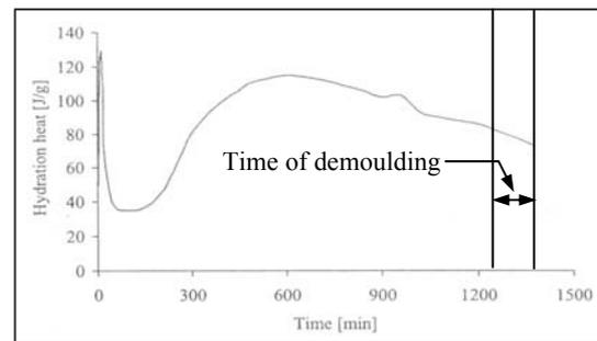
Fig. 3 A typical of heat liberation (J/g) from hydration reactions [16]
