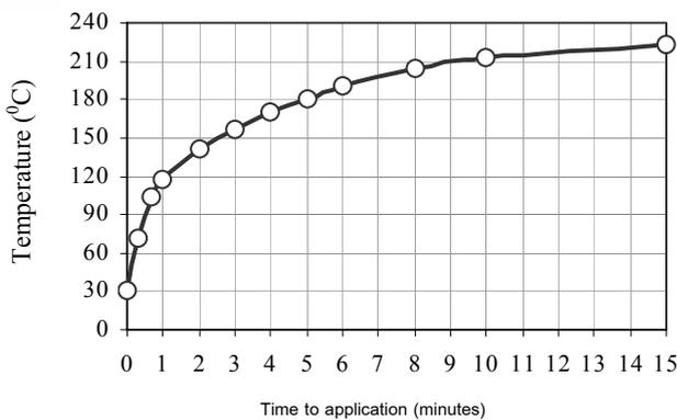
Fig. 8 Temperature rise between microwave heating
