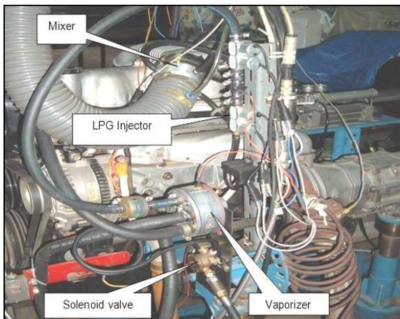
Figure 6 Arrangement of LPG injection system
