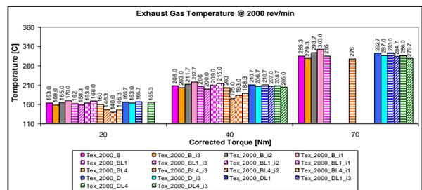
Figure 26 Exhaust gas temperature with different modes of operation and injection timing, at 2000 rev/min. [15]
