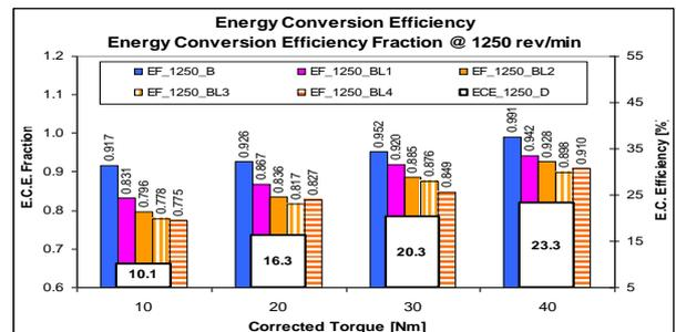
Figure 14 ECE @ 1250 rev/min, PME & LPG-PME modes
