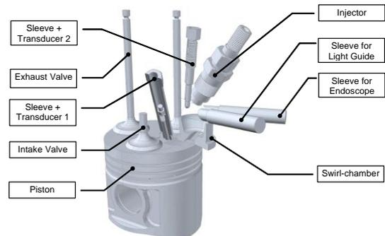
Figure 3 Setup of transducers for cylinder pressure measurement.
