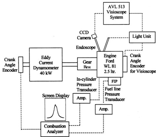
Figure 4 Schematic arrangement of experimental set up
