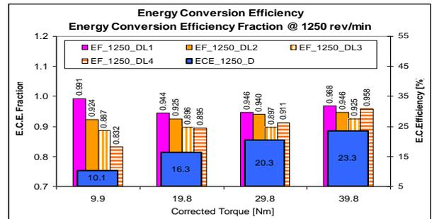
Figure 12 ECE # 1250 rev/min, diesel and LPG-diesel modes
