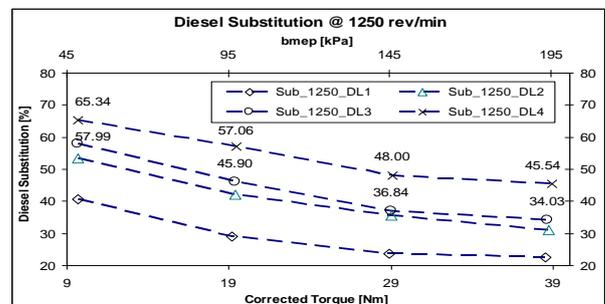
Figure 8 Diesel substitution # 1250 rev/min, LPG-diesel modes
