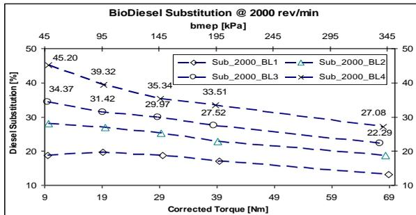
Figure 11 Substitution @ 2000 rev/min LPG-PME modes
