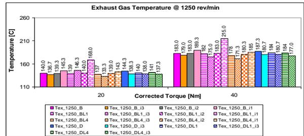
Figure 25 Exhaust gas temperature with different modes of operation and injection timing, at 1250 rev/min. [15]
