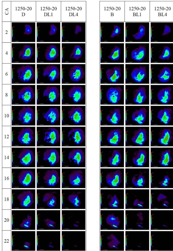
Figure 20 Images of soot concentration distribution at 1250 rev/min, 20 Nm (modes: D, DL1, DL4, B, BL1, and BL4). [15]
