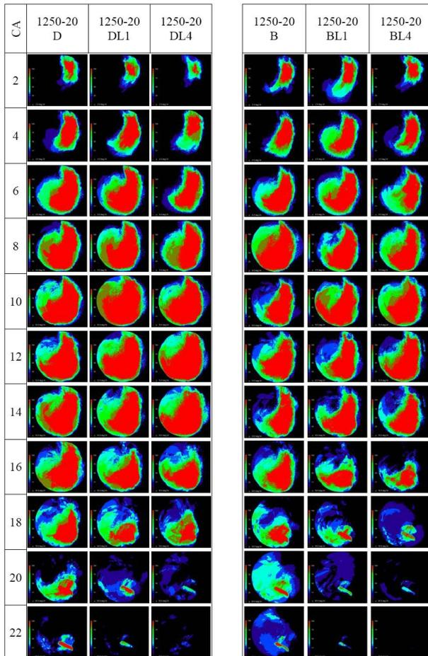
Figure 18 Images of flame probability distribution at 1250 rev/min, 20 Nm (modes: D, DL1, DL4, B, BL1, and BL4) [15]
