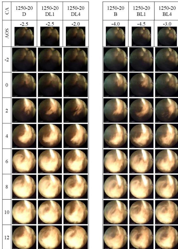
Figure 16 Sequential images of combustion process with cool light at 1250 rev/min, 20 Nm (modes: D, DL1, DL4, B, BL1, and BL4) [15]
