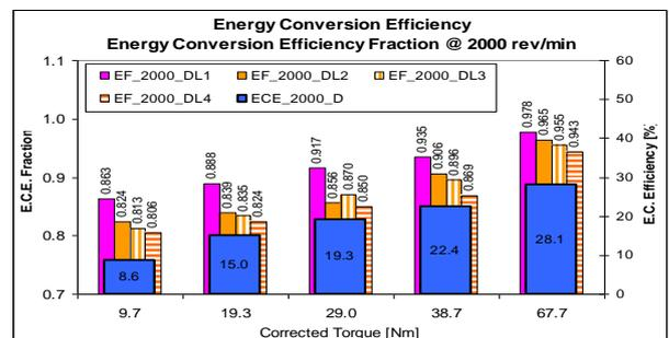
Figure 13 ECE # 2000 rev/min, diesel and LPG-diesel modes
