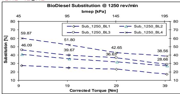
Figure 10 Substitution @ 1250 rev/min, LPG-PME modes
