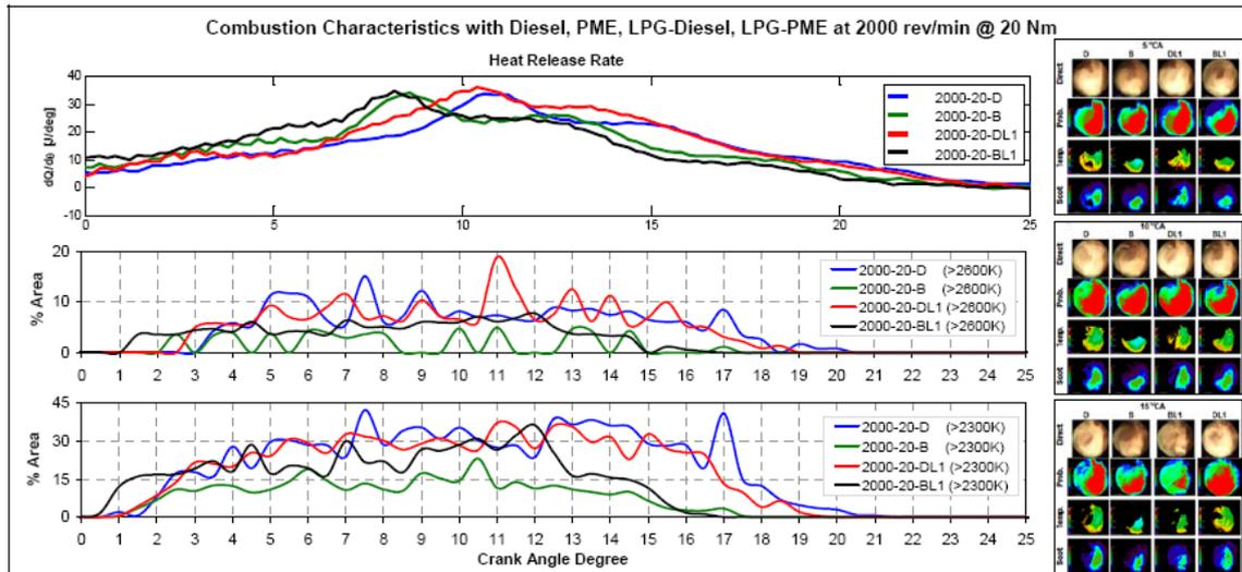
Figure 22 HRR and area of flame temperature above 2300 and 2600K at 2000 rev/min, 20Nm, (mode D, DL1, B, and BL1) [15]
