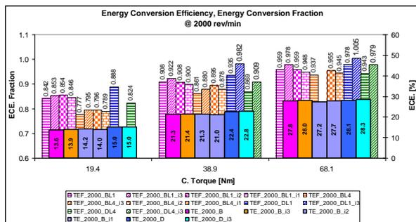
Figure 24 ECE and ECE fraction with different modes of operation and injection timing, at 2000 rev/min. [15]
