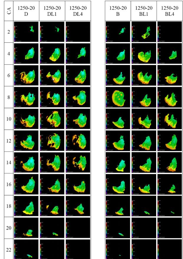
Figure 19 Images of flame temperature distribution at 1250 rev/min, 20 Nm (modes: D, DL1, DL4, B, BL1, and BL4) [15]
