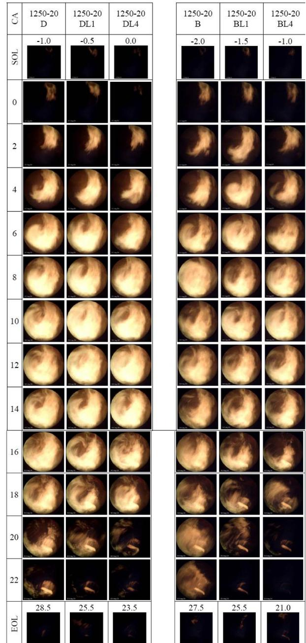
Figure 17 Sequential images of combustion process at 1250 rev/min, 20 Nm (modes: D, DL1, DL4, B, BL1, and BL4) [15]
