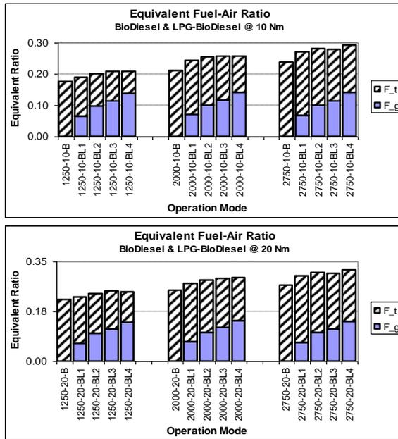
Figure 7  $\phi$  of the premixed charge and total equivalence ratio
