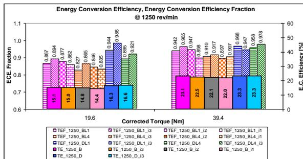
Figure 23 ECE and ECE fraction with different modes of operation and injection timing, at 1250 rev/min. [15]
