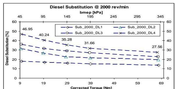
Figure 9 Diesel substitution # 2000 rev/min, LPG-diesel modes
