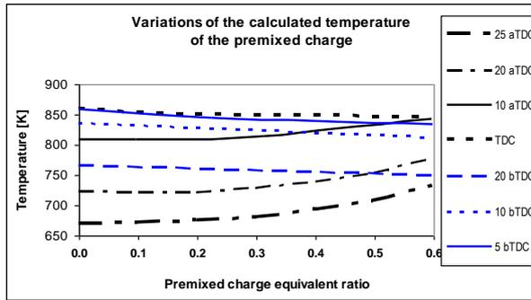
Figure 1 Variations of calculated CH<sub>4</sub>-air charge temperature in compression and expansion strokes of a motored engine without pilot injection, (reproduced from [6])
