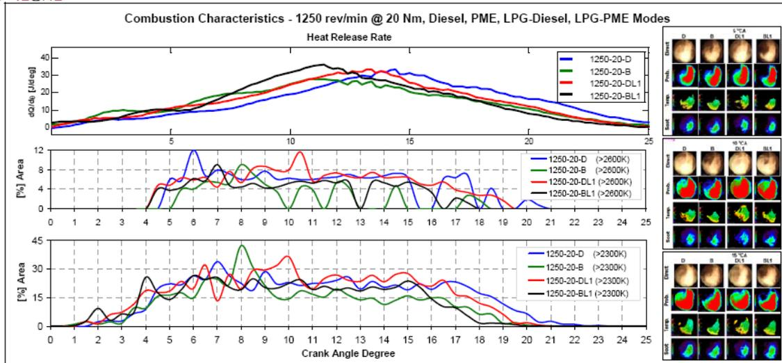
Figure 21 HRR and area of flame temperature above 2300 and 2600K at 1250 rev/min, 20Nm, (mode D, DL1, B, and BL1) [15]
