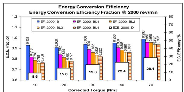
Figure 15 ECE @ 2000 rev/min, PME & LPG-PME modes
