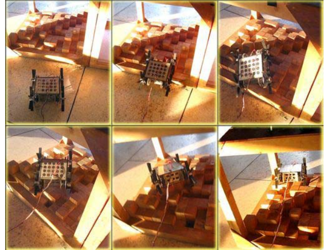
Figure 11. Six-spoke wheel traversing across Robocup Rescue site
