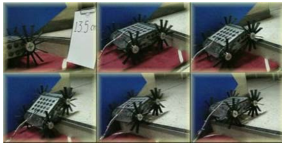
Figure 9. Twelve-spoke wheel climbing up the stairs
