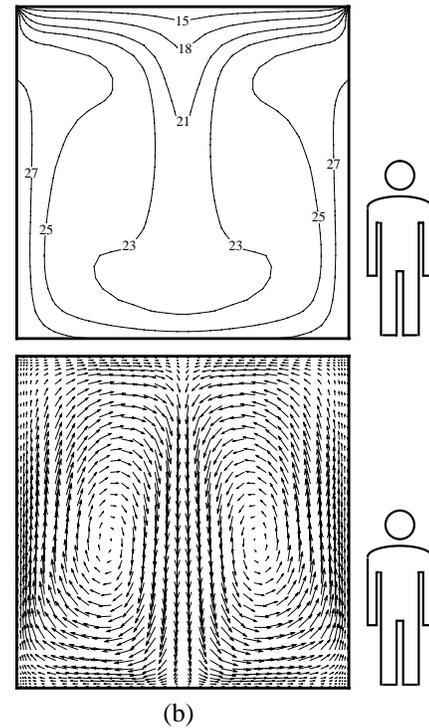
Figure 4. Temperature and velocity profiles for the square room (a) Floor cooling at  $T_{RCP} = 10^\circ\text{C}$  (b) Ceiling cooling at  $T_{RCP} = 13^\circ\text{C}$  (c) Wall cooling at  $T_{RCP} = 13^\circ\text{C}$
