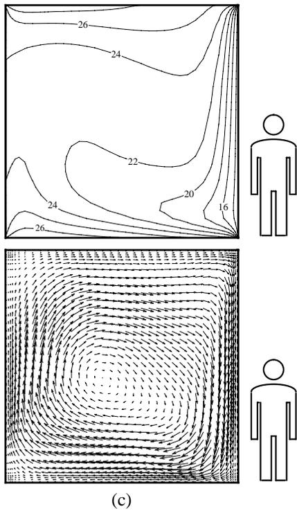
Figure 4. Temperature and velocity profiles for the square room (a) Floor cooling at  $T_{RCP} = 10^\circ\text{C}$  (b) Ceiling cooling at  $T_{RCP} = 13^\circ\text{C}$  (c) Wall cooling at  $T_{RCP} = 13^\circ\text{C}$  (Cont'd)
