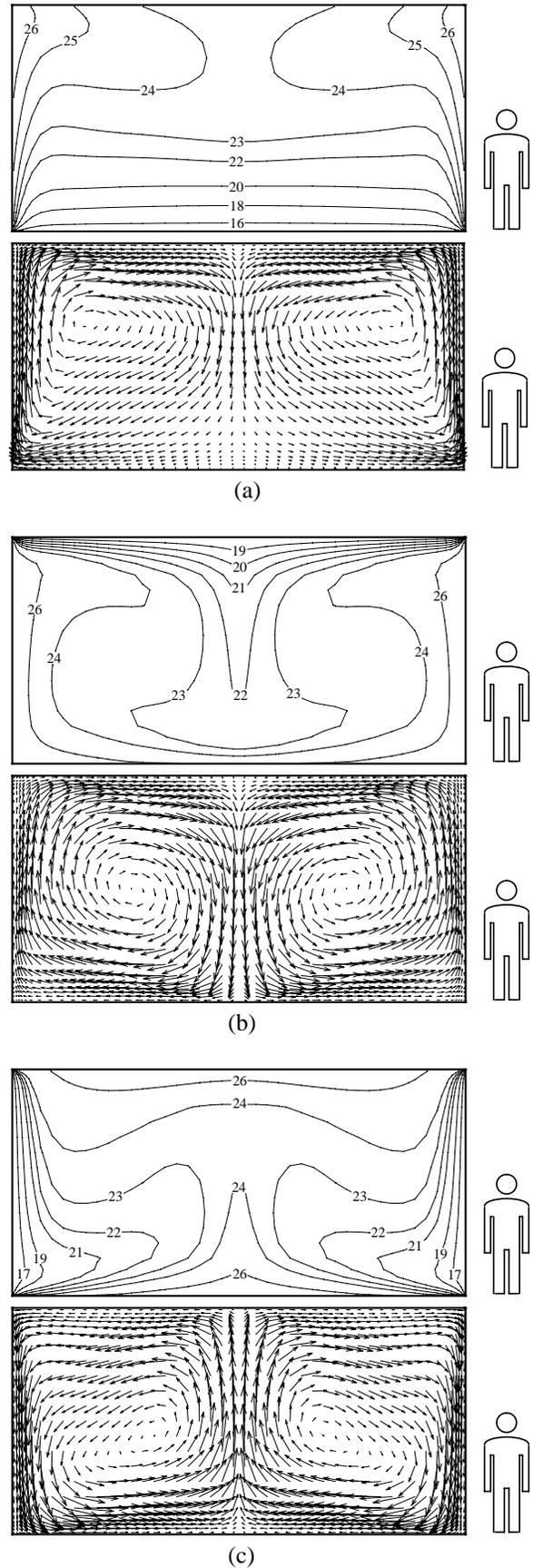
Figure 6. Temperature and velocity profiles for the hall (a) Floor cooling at  $T_{RCP} = 15^\circ\text{C}$  (b) Ceiling cooling at  $T_{RCP} = 18^\circ\text{C}$  (c) Wall cooling at  $T_{RCP} = 15^\circ\text{C}$
