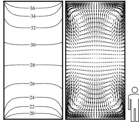
Figure 8. Temperature and velocity profiles for the high rise hall with the floor cooling at  $T_{RCP} = 18^{\circ}\text{C}$
