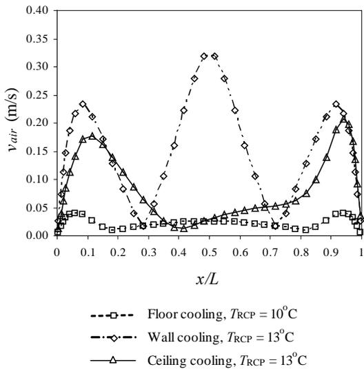
Figure 5. Absolute velocity at half height for the square room
