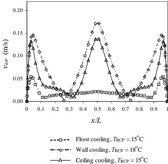
Figure 7. Absolute velocity at half height for the hall
