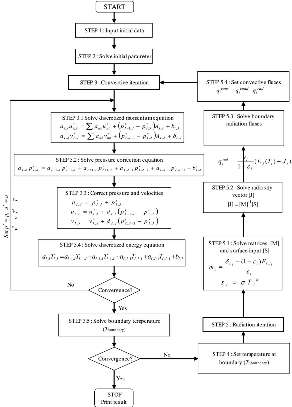
Figure 3. Combined convection and radiation computation flow chart
