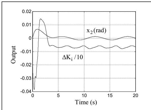
Fig. 2 Response of the integral gain scheduling PID system
