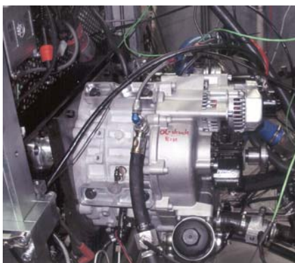
Figure 1. The Wankel engine on an engine test-bed
