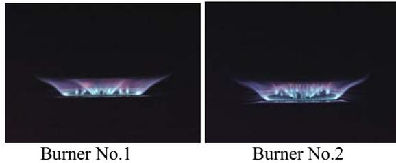
Fig. 8. Typical impinging flame. (radial flow)
