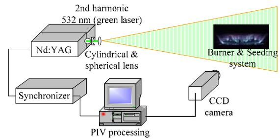
Fig. 2. Test burner and PIV setup.
