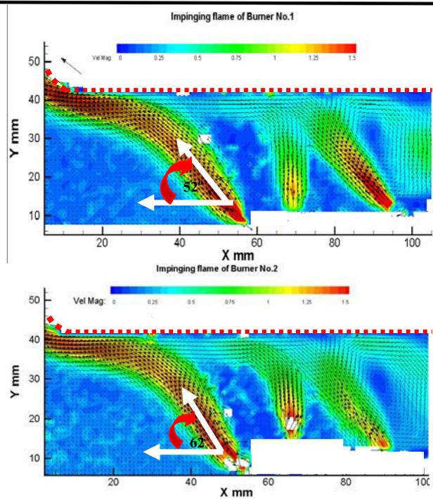
Fig. 9. Typical velocity field of impinging flame for burner No1 (top) and burner No2 (below).
