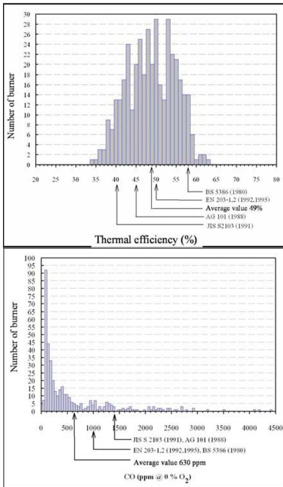
Fig. 4.  $\eta$  (above) and CO emission (below) of LPG cooking burners in Thailand.
