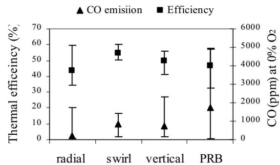
Fig. 6. Thermal efficiency and CO emission of tested cooking burners.
