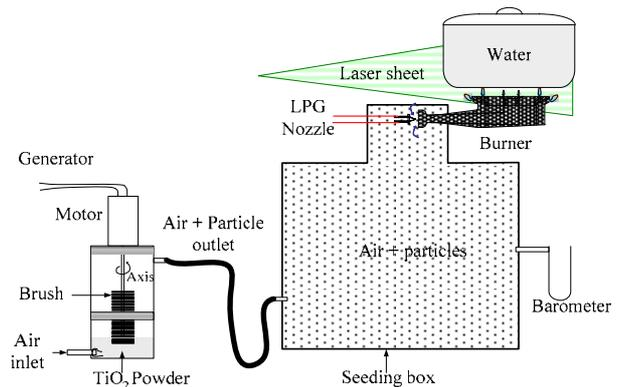
Fig. 3. Schematic of the seeding systems.
