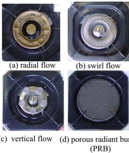
Fig. 1. Photographs of tested cooking burners.
