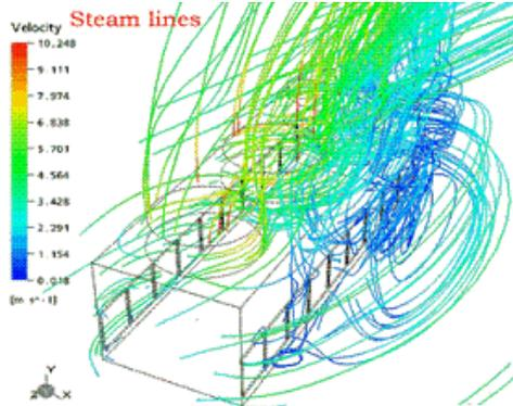
Fig. 7 Streamlines around the cooling tower
