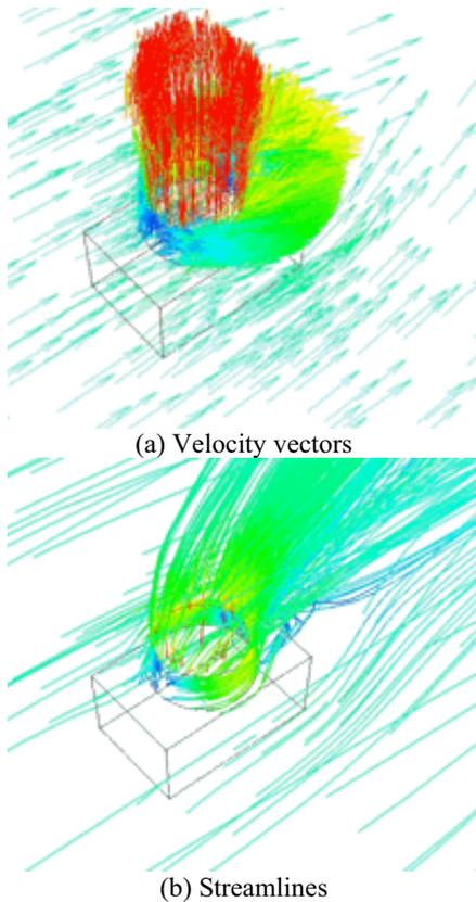
Fig 4 Flow around the cooling tower when wind flows directly to the inlet air opening
