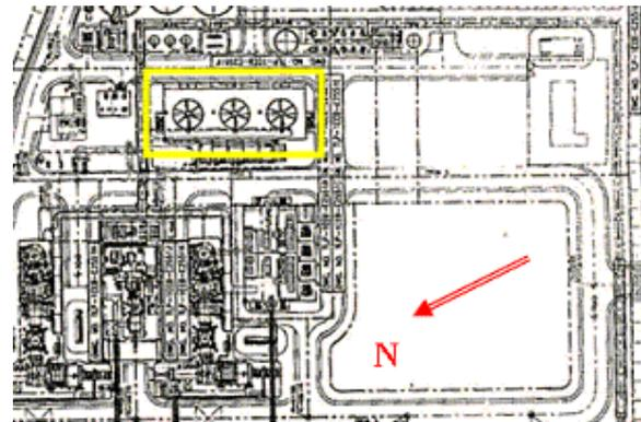
Fig 5 Installation plane of the 3 cells cooling tower
