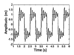
Fig. 9 Perturbed plant with the input shaper: (dash) reference r, (solid) output y.
