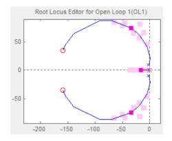
Fig. 5 Root locus with a PID controller.
