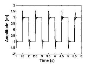
Fig. 7 Nominal plant without the input shaper: (dash) reference r, (solid) output y.
