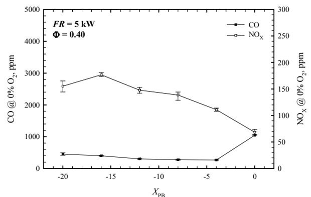
Fig. 6 Influence of  $X_{PB}$  on CO and NO<sub>x</sub> emissions
