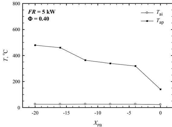
Fig. 7 Influence of  $X_{PB}$  on preheated temperature
