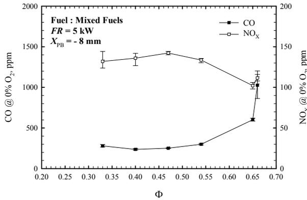
Fig. 4 Influence of  $\Phi$  on CO and NO<sub>x</sub> emissions
