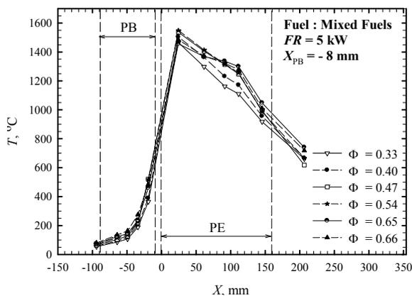
Fig. 3 Influence of  $\Phi$  on temperature profile
