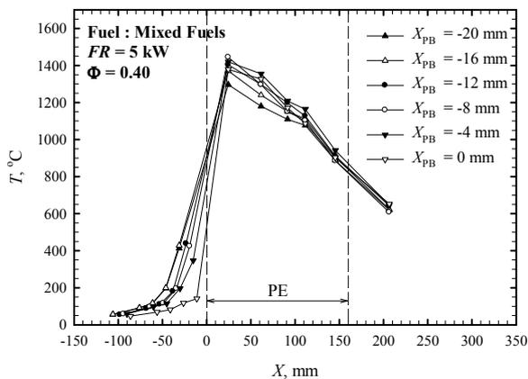
Fig. 5 Influence of  $X_{PB}$  on temperature profile
