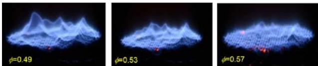
Fig. 4 The side-view photographs of cellular flames at  $\phi=0.49$ ,  $\phi=0.53$  and  $\phi=0.57$ .
