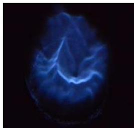
Fig. 6 The top-view photographs of blew off flame at  $\phi=0.45$ .
