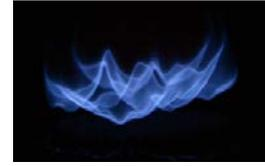
Fig. 7 The side-view photographs of blew off flame at  $\phi=0.45$ .
