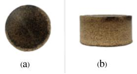
Fig. 4 Photos of the example biocoke prepared from rubberwood sawdust by using used coffee ground as a binder: (a) top view and (b) side view
