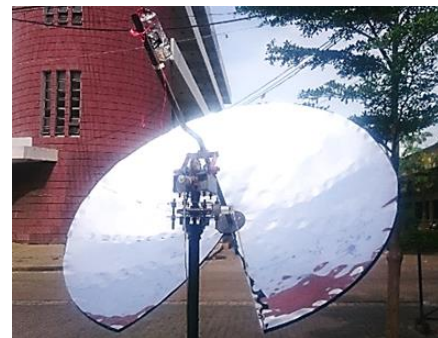
Fig. 16 the material on solar collector was PET aluminum
