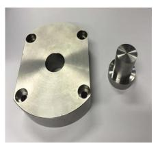
Fig.3 Mold for compressing bamboo powder sample
