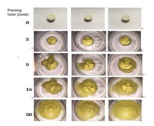
Fig.4 Water swelling properties investigation with 3 different mold pressure
