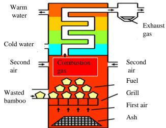
Fig.8 Concept model of the proposed boiler
