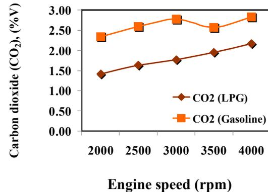
Fig. 11 Relationship of CO<sub>2</sub> and engine speed for LPG and Gasoline
