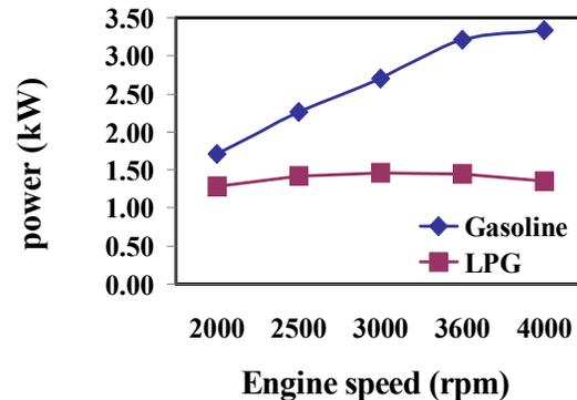
Fig. 3 Net output power at different engine speeds for LPG and gasoline
