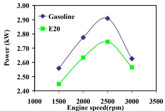
Fig. 4 Net output power at different engine speeds for gasoline and E20
