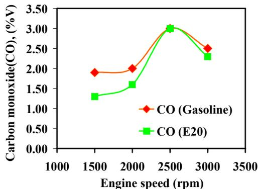
Fig. 10 Relationship of carbon monoxide (CO) and engine speed of gasoline and E20.
