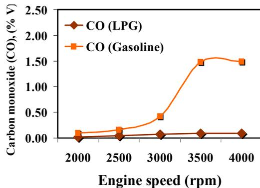
Fig. 9 Relationship of CO and engine speed for LPG and gasoline
