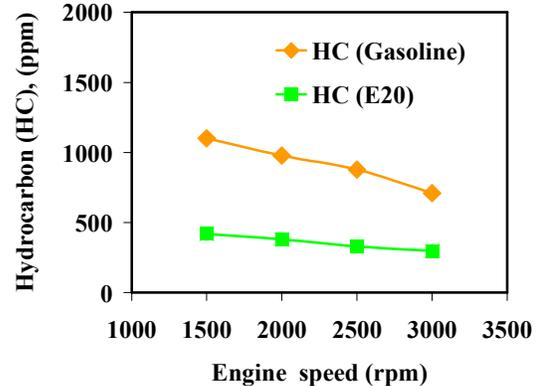
Fig. 14 Hydrocarbon (HC) at different engine speeds of gasoline and E20.
