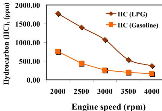
Fig. 13 Relationship of HC and engine speed for LPG and
