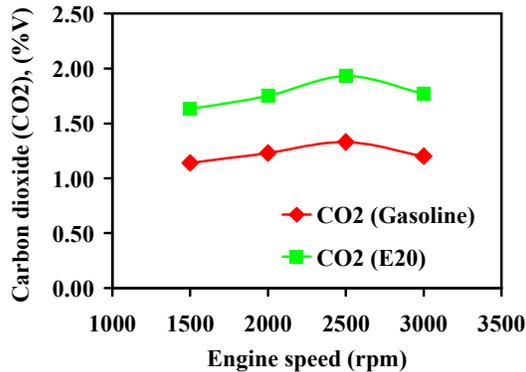
Fig. 12 Relationship of carbon dioxide (CO<sub>2</sub>) and engine speed of gasoline and E20.
