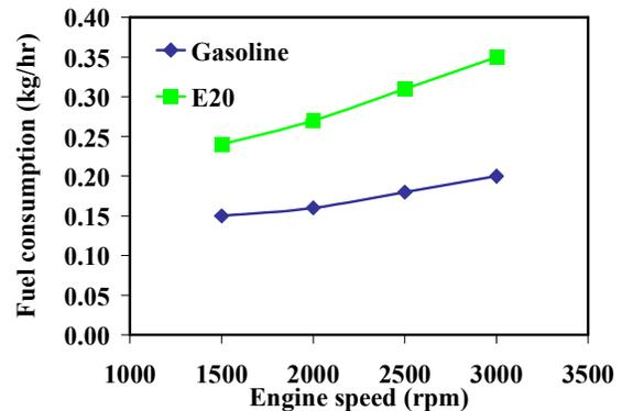
Fig. 8 Fuel consumption of gasoline and E20 at different engine speeds
