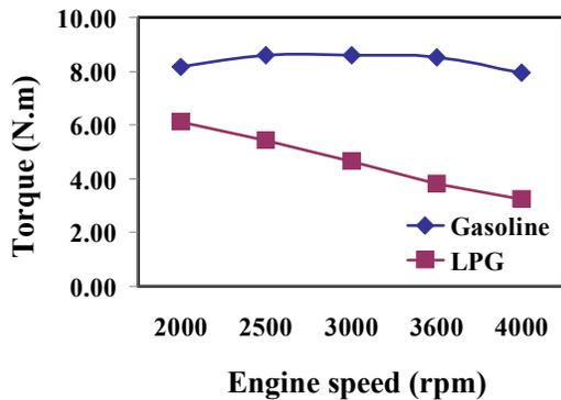
Fig. 5 Relationship of output torque at different engine speeds for LPG and gasoline
