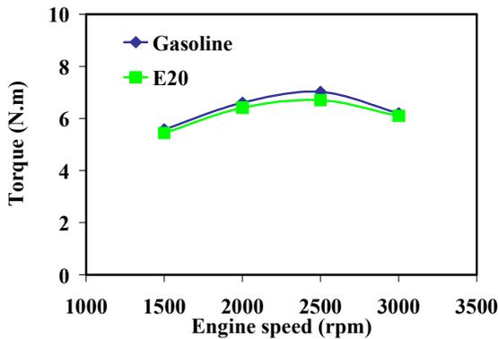
Fig. 6 Relationship of output torque at different engine speeds for E20 and gasoline
