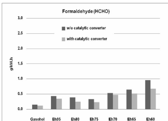
Fig. 9. Formaldehyde from combustion of hydrous ethanol with various water contents at 3300 rpm, load 4 kW and stoichiometric A/F.
