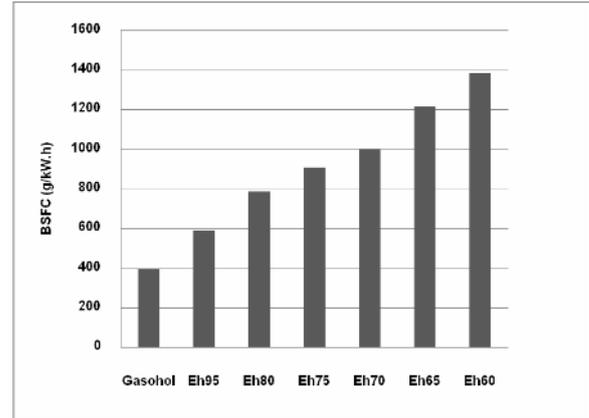
Fig. 3. Brake specific fuel consumption with various water contents in ethanol at 3300 rpm, 4 kW load and stoichiometric A/F ( $\lambda=1$ ).
