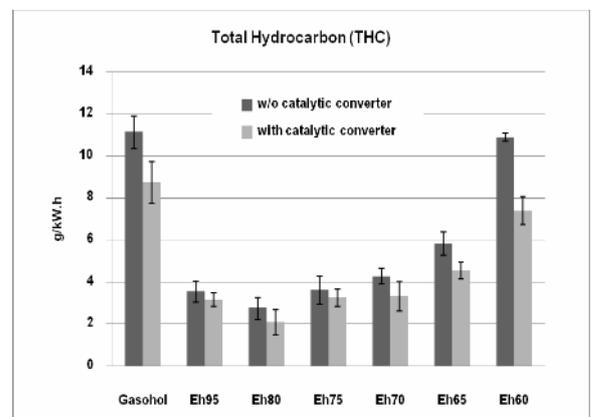
Fig. 8. Total hydrocarbon from combustion of hydrous ethanol with various water contents at 3300 rpm, load 4 kW and stoichiometric A/F.
