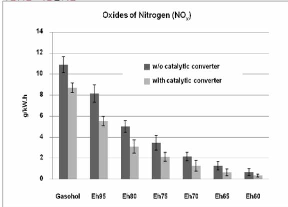
Fig. 5. Oxides of nitrogen from combustion of hydrous ethanol with various water contents at 3300 rpm, load 4 kW and stoichiometric A/F.
