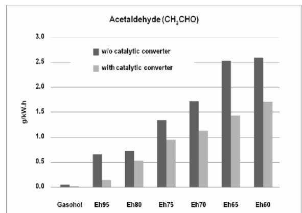
Fig. 10. Acetaldehyde from combustion of hydrous ethanol with various water contents at 3300 rpm, load 4 kW and stoichiometric A/F.
