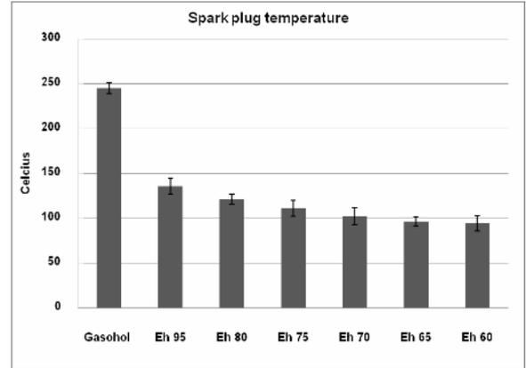
Fig. 6. Spark plug temperature at 3300 rpm, load 4 kW and stoichiometric A/F.
