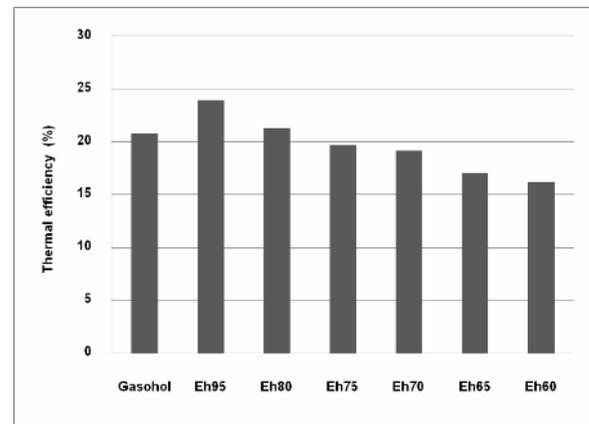
Fig. 4 Thermal efficiency with various water contents in ethanol at 3300 rpm, 4 kW load and stoichiometric A/F ( $\lambda=1$ ).
