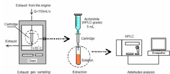
Fig. 2 schematic diagram of exhaust gas sampling for aldehyde analysis
