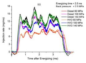
Fig. 6(c) Injection rate profile of diesel and HVO and injection pressure of 60, 100 and 140 MPa
