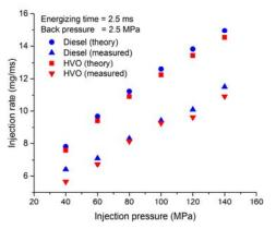
Fig.7 Measured injection rate and various injection pressure
