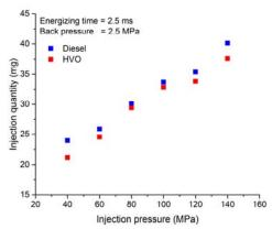
Fig. 8 Injection quantity and various injection pressure
