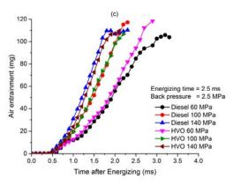
Fig. 9(c) Air entrainment of diesel and HVO and injection pressure of 60, 100 and 140 MPa
