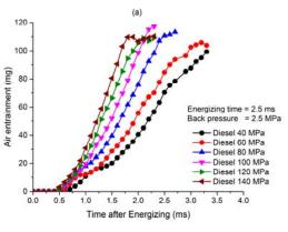
Fig. 9(a) Air entrainment of diesel and various injection pressure
