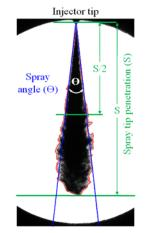
Fig. 2 Definition of fuel spray injection
