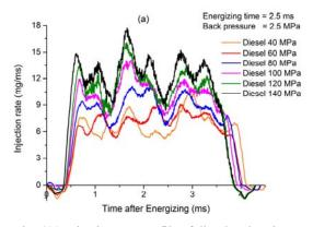
Fig. 6(a) Injection rate profile of diesel and various injection pressure
