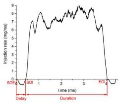
Fig. 1 Definition typical injection process
