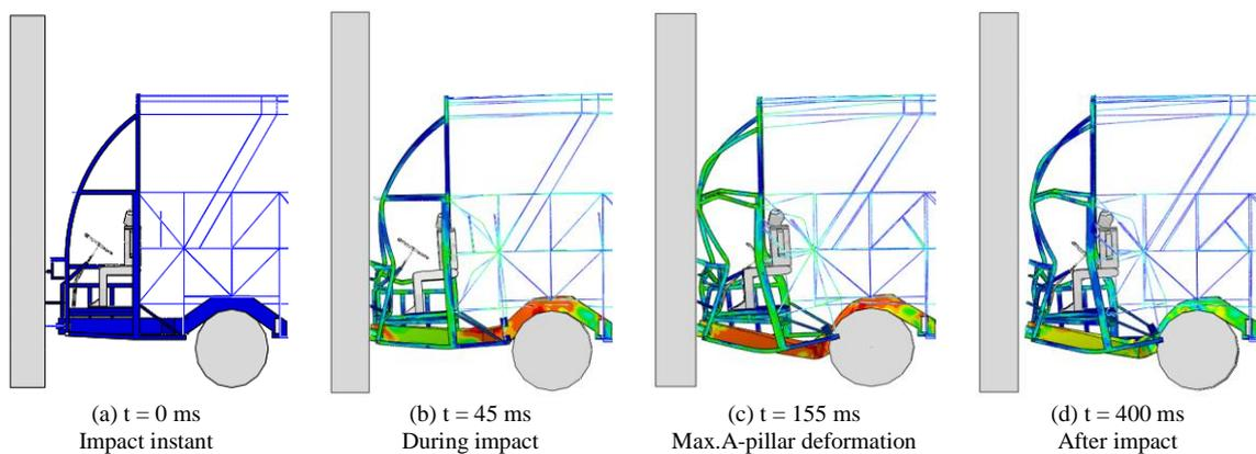
Fig. 8 Deformation shapes at different time instances of FMVSS-208
