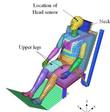
Fig. 6 Hybrid III 50<sup>th</sup> percentile driver dummy model
