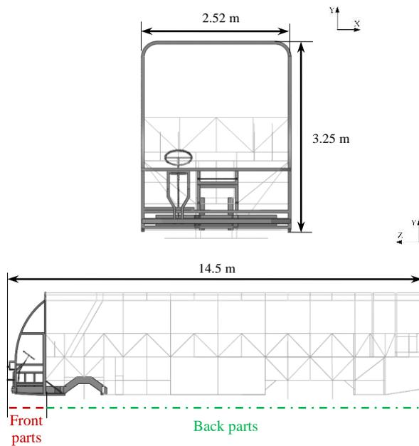
Fig. 3 Bus structure model
