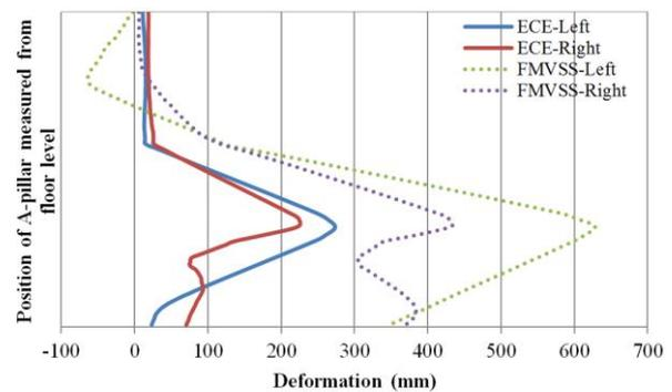
Fig. 9 Deformation of A-pillar after impact
