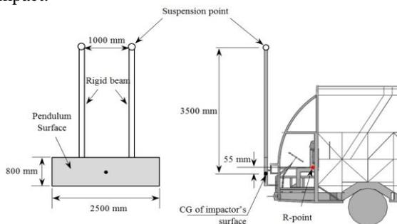
Fig. 1 Front impact test according to ECE-R29 Test A
