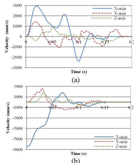
Fig. 12 Imposed velocity of (a) ECE-R29 Model (b) FMVSS 208 Model
