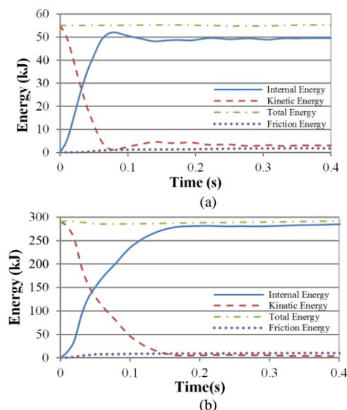
Fig. 11 Energy plot during impact simulation (a) ECE-R29 regulation and (b) FMVSS-208 regulation
