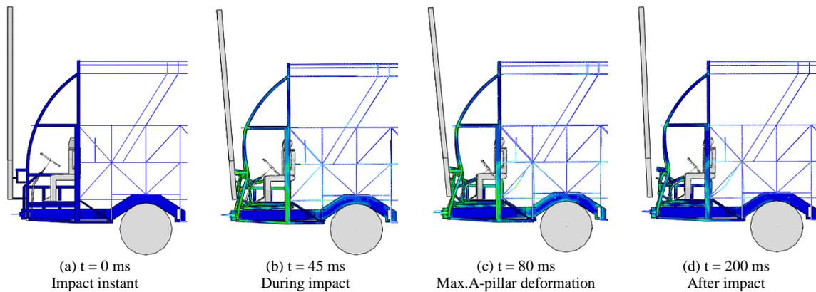
Fig. 7 Deformation shapes at different time instances of ECE-R29
