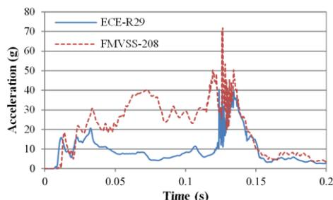
Fig. 13 Head acceleration in term g during impact
