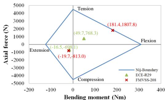
Fig. 14 Nij-boundary for axial force and bending moment
