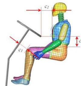
Fig. 10 Clearances between driver and steering system
