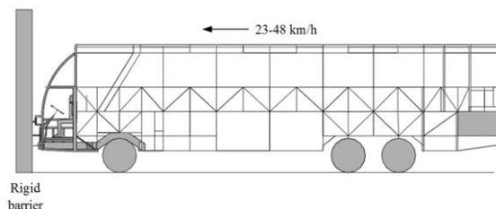
Fig. 2 Head-on full frontal fixed barrier
