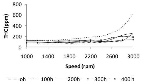
Fig.13 THC emission at various engine speeds
