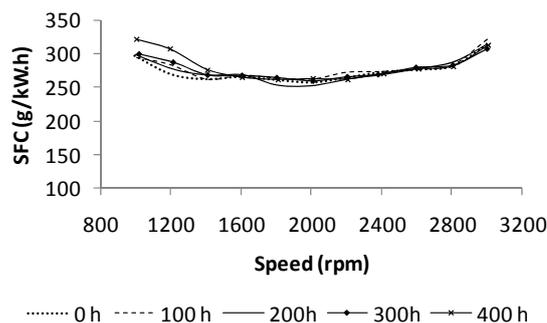
Fig.5 Fuel consumption at various engine speeds
