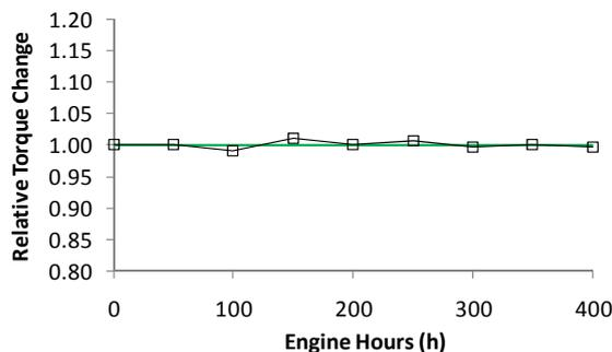
Fig.4 Maximum engine torque change relative to prior condition at 0 hour
