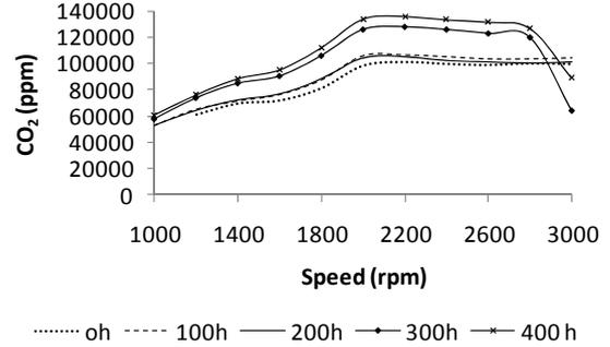
Fig.11 CO<sub>2</sub> emission at various engine speeds
