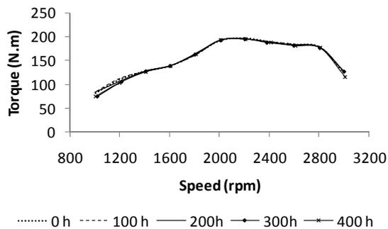
Fig.3 Engine torque at various engine speeds
