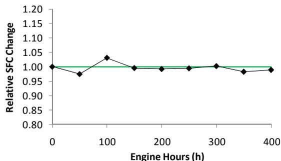
Fig.6 Optimal specific consumption change relative to prior condition at 0 hour
