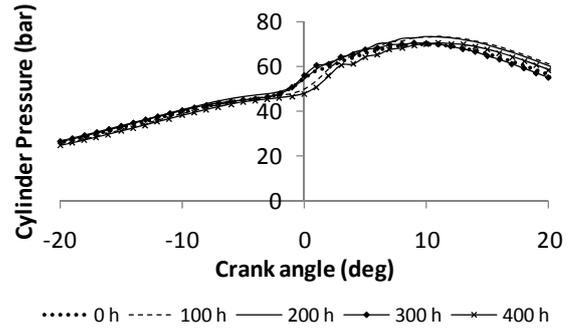
Fig.8 Cylinder pressure at 2200 rpm at various engine hours
