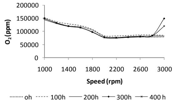
Fig.14 O<sub>2</sub> at various engine speeds
