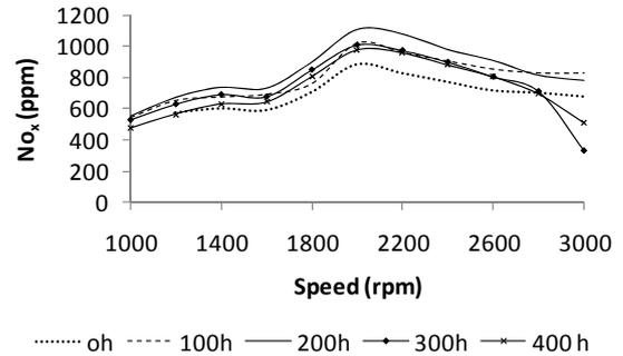
Fig.12 NO<sub>x</sub> emission at various engine speeds
