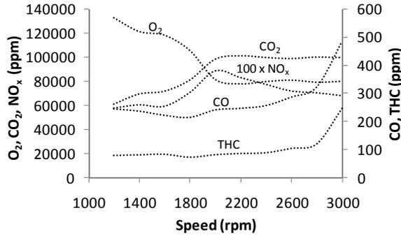
Fig.9 Exhaust emissions at the beginning of the test (0 hour)
