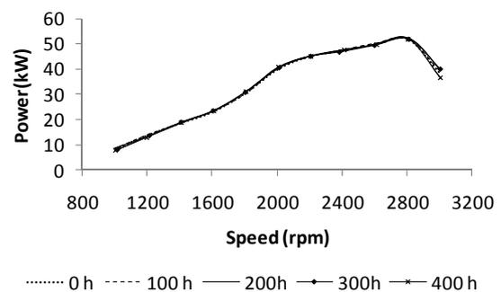
Fig.2 Engine power at various engine speeds
