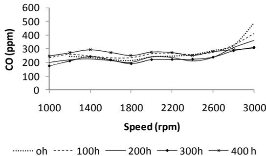
Fig.10 CO emission at various engine speeds
