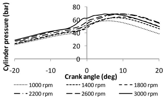
Fig.7 Cylinder pressure at various speed at 0 hour
