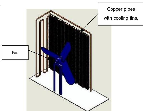
Figure 4 Biogas cooling System
