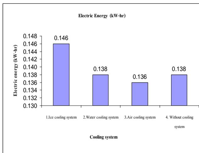
Figure 8 Comparison of electric energy consumption
