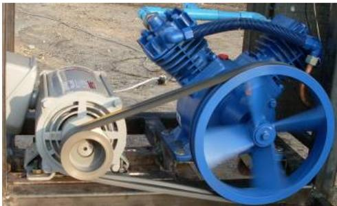
Figure 2 Biogas compressor and motor
