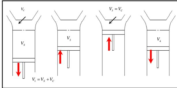
Figure 1 Operation of the piston
