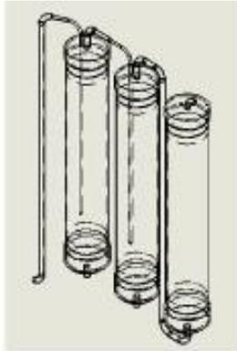
Figure 3 Biogas Scrubbing System
