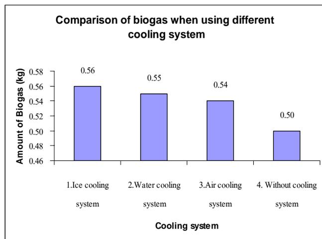
Figure 7 Comparison of biogas when using different cooling system
