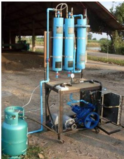
Figure 5 Biogas Compression Systems
