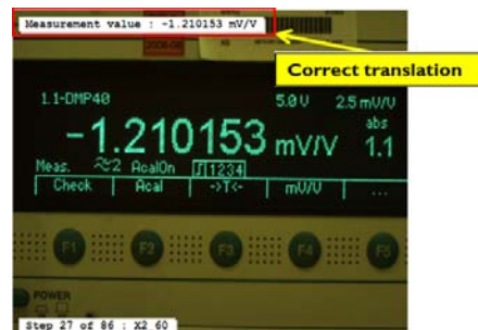
Fig.11. The translation of the image to measurement data
