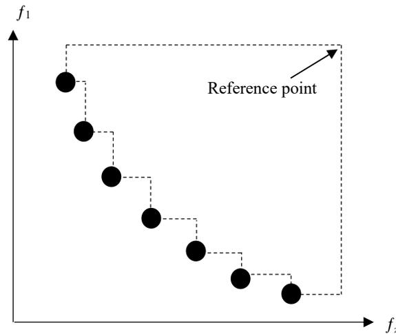
Fig. 8 Area to calculate  $HV$  [25]
