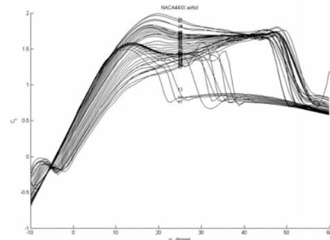
Fig. 6  $C_l$  with angle of attack of NACA44XX
