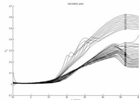
Fig. 7  $C_d$  with angle of attack of NACA44XX
