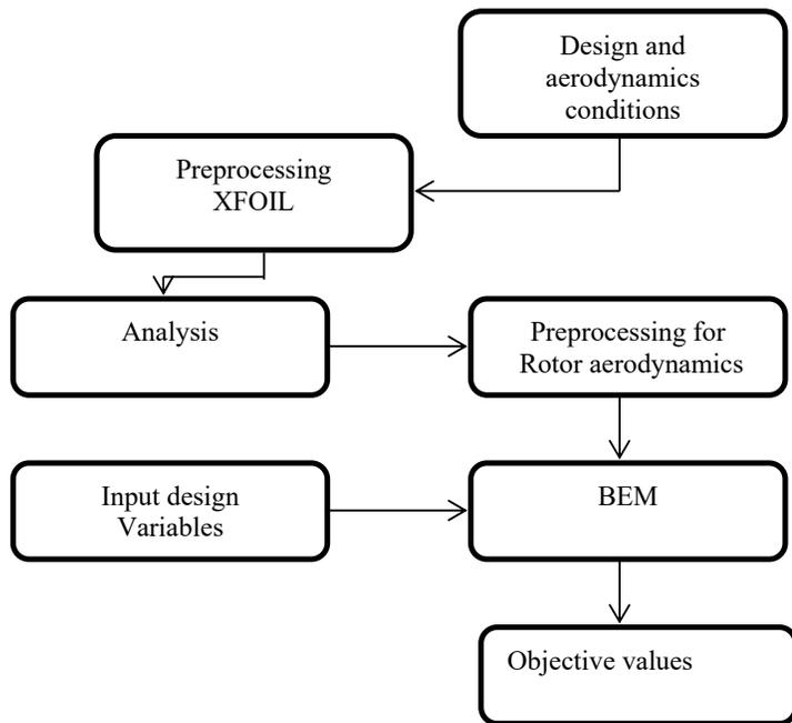
Fig. 5 Flowchart for function evaluation
