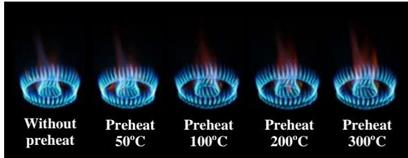
Fig. 6 Effecting of primary air preheat on flame structure at  $q = 8.41$  kW
