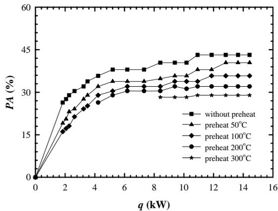
Fig. 2 Typical primary aeration of a self-aspirating burner
