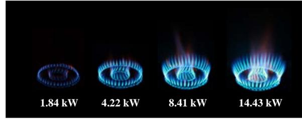
Fig. 5 Effecting of heat input on flame structure for without preheat case
