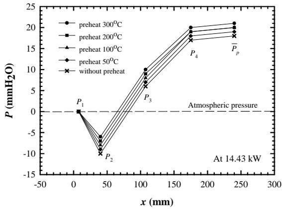
Fig. 4 Effecting of primary air preheat on pressure drop along a self-aspirating burner
