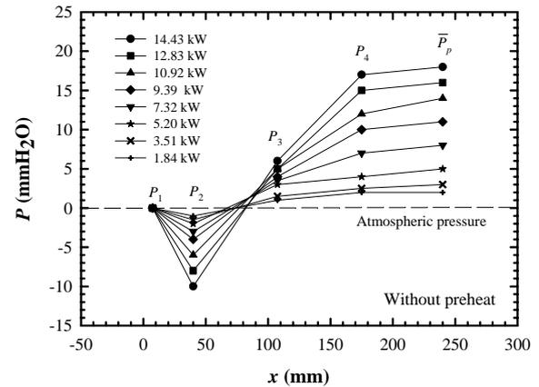
Fig. 3 Effecting of heat input on pressure drop along a self-aspirating burner
