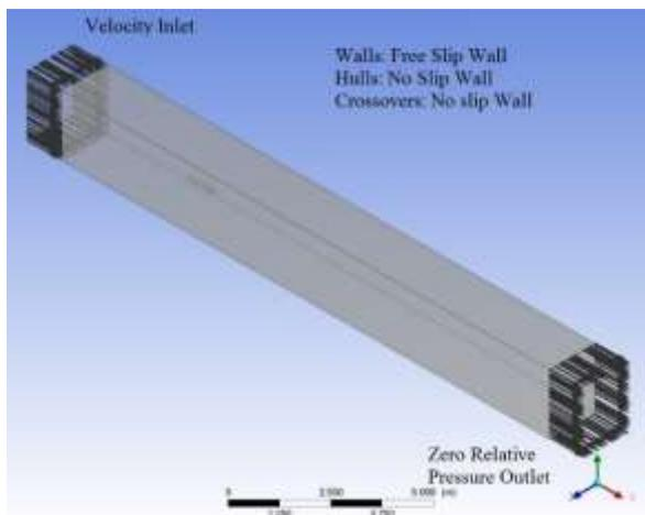
Figure 4: Fluid domain and boundary condition
