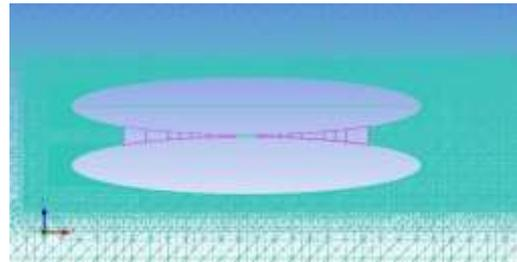
Figure 5: Fine mesh set on ZX plane at  $Y = 0$  from the centerline with the fluid flow from left to right
