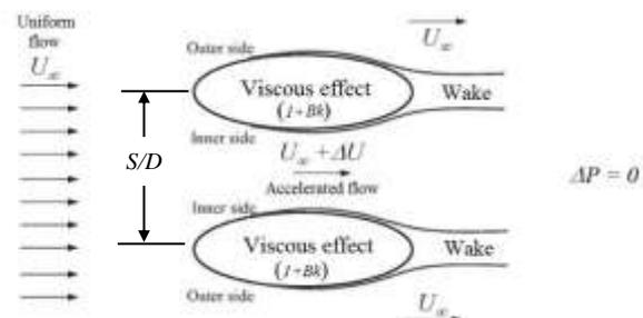
Figure 1: Flow past twin hulls in parallel configuration
