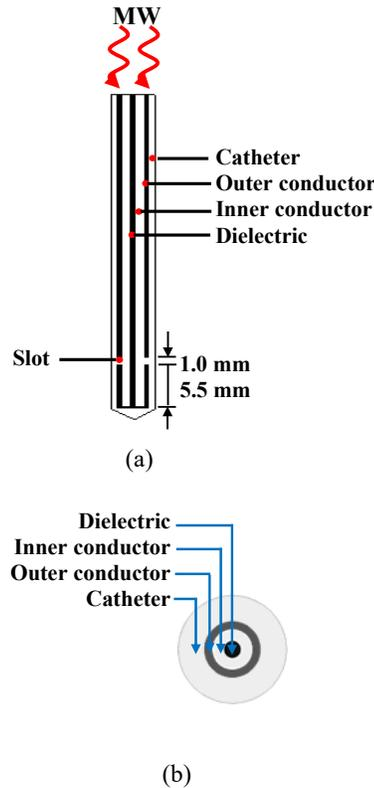
Fig. 1 Schematic diagram of a single-slot microwave antenna (a) Axial schematic of a single-slot microwave antenna and (b) Cross section of the single-slot microwave antenna
