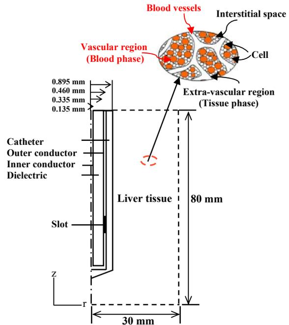
Fig. 2 Axially symmetric model geometry
