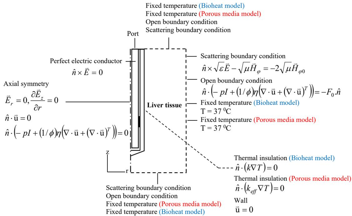
Fig. 3. Boundary conditions for analysis
