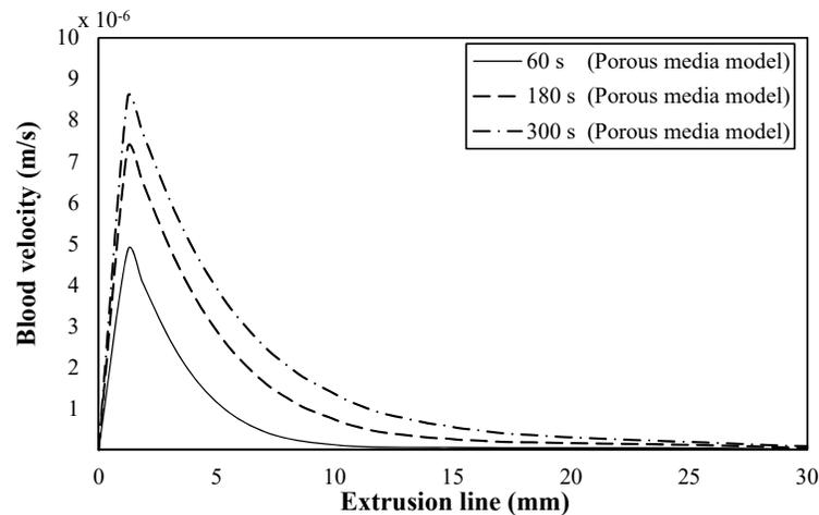
Fig. 10 The blood velocity distribution in liver tissue along the extrusion line based on a frequency of 2.45 GHz, input microwave power of 10 W and tissue porosity of 0.6 at various times.
