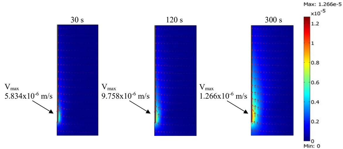
Fig. 9 The blood velocity profile in liver tissue at various time based on a frequency of 2.45 GHz, input microwave power of 10 W and tissue porosity of 0.6 calculated using the porous media model
