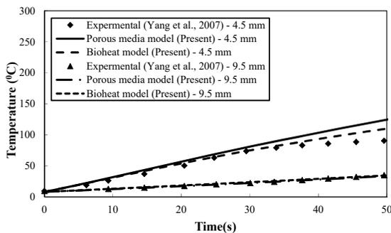
Fig. 6 The validation results of the liver tissue temperature from the porous model and bioheat model with the liver tissue temperature from experimental results, against Yang et al. [11].
