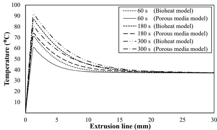
Fig. 8 The temperature distribution in liver tissue along the extrusion line based on a frequency of 2.45 GHz, input microwave power of 10 W and tissue porosity of 0.6 at various times.
