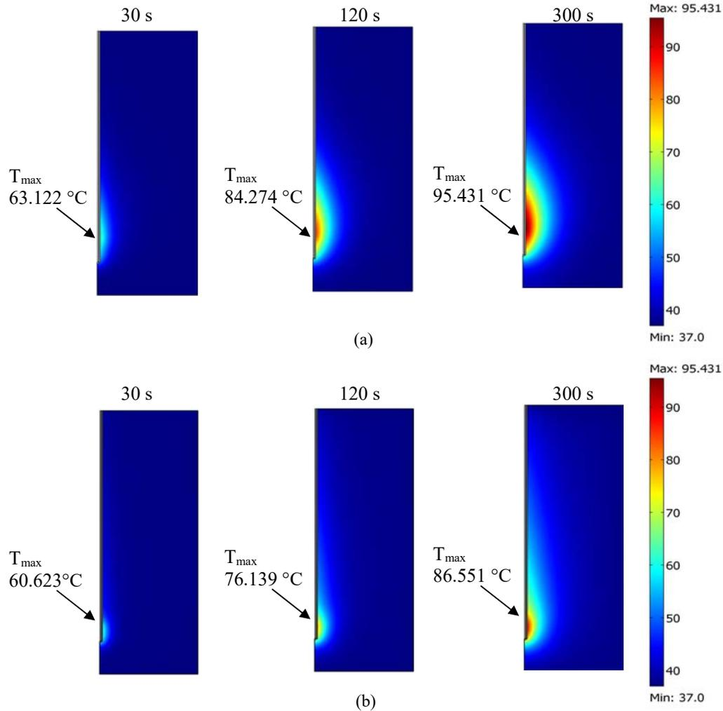
Fig. 7. The temperature profile in liver tissue at various time based on a frequency of 2.45 GHz, input microwave power of 10 W and tissue porosity of 0.6 calculated using; (a) bioheat model and (b) porous media model.
