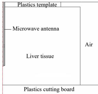
Fig. 4 Geometry of the validation model obtained by Yang et al. [11]
