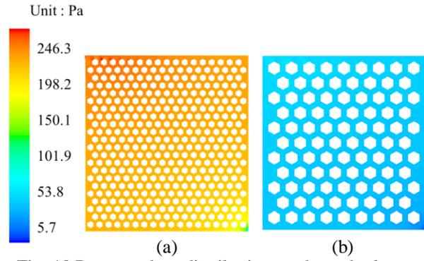
Fig. 10 Pressure drop distribution on the cathode gas diffusion layer and the gas flow channel interface a) new honeycomb and b) previous honeycomb design at 0.8 A cm<sup>-2</sup>
