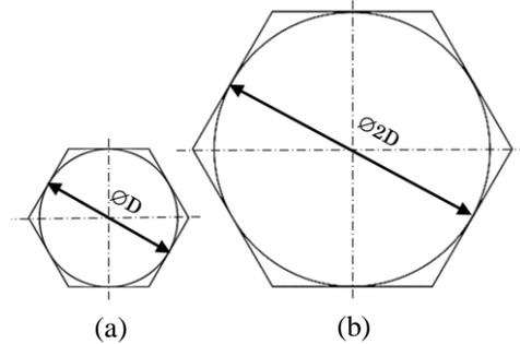
Fig. 3 Hexagon land size a) new honeycomb and b) previous honeycomb design
