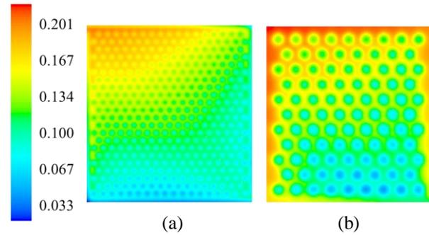
Fig. 7 Oxygen mass fraction distribution on the cathode catalyst and the gas diffusion layer interface of a) new honeycomb and b) previous honeycomb design at 0.8 A cm<sup>-2</sup>
