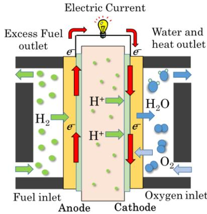
Fig. 1 The schematic shows how polymer electrolyte fuel cell works [3]
