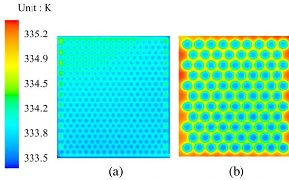
Fig. 8 Temperature distribution on the cathode membrane and the catalyst interface of a) new honeycomb and b) previous honeycomb design at 0.8 A cm<sup>-2</sup>
