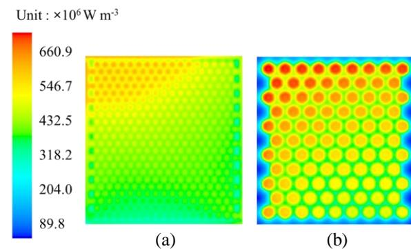
Fig. 9 Reaction heat source distribution on the cathode membrane and the catalyst interface of a) new honeycomb and b) previous honeycomb design at 0.8 A cm<sup>-2</sup>
