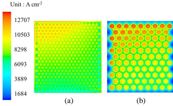
Fig. 5 Current density distribution on the cathode catalyst and the gas diffusion layer interface of a) new honeycomb and b) previous honeycomb design at 0.8 A cm<sup>-2</sup>
