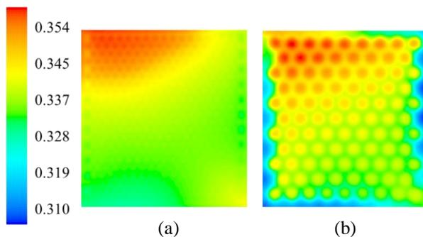
Fig. 6 Hydrogen mass fraction distribution on the anode catalyst and the gas diffusion layer interface of a) new honeycomb and b) previous honeycomb design at 0.8 A cm<sup>-2</sup>
