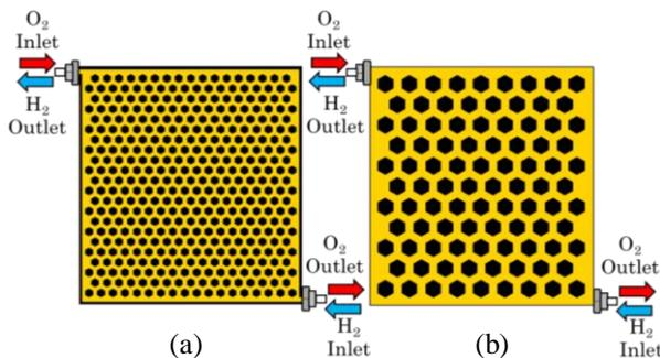
Fig. 2 The schematic illustration of the flow fields simulated in this work a) new honeycomb and b) previous honeycomb (→) Anode and (→) Cathode flow directions
