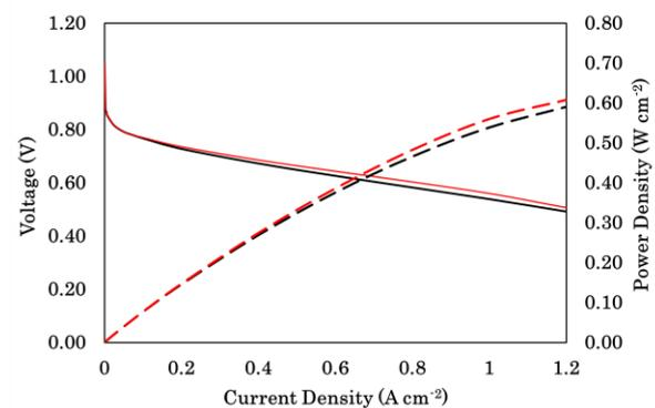
Fig. 4 The IV performance (solid lines) and power curves (dashed lines) of two different flow field designs. (—) New honeycomb and (—) previous honeycomb design.
