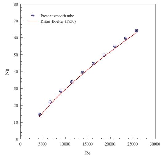
Fig. 3. Confirmatory test of  $Nu$  of plain tube.
