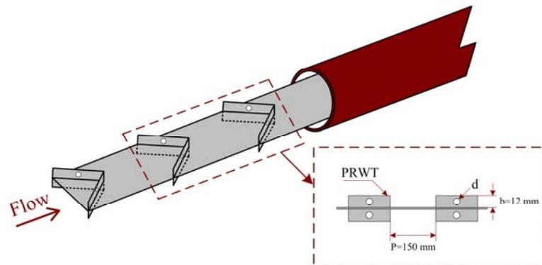
Fig. 2 Test section with 45° PRWT inserts.
