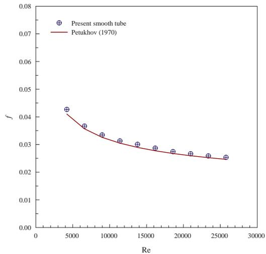
Fig. 4. Confirmatory test of  $f$  of plain tube.
