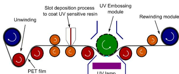
Fig. 2 Schematic of roll-to-roll fabrication setup for patterning polymer films
