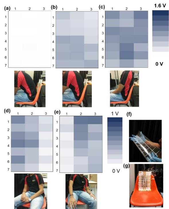
Fig. 7. Heat map of the sensor array for different posture when array assembled on back of chair. (a) Without touching the sensor array, (b) partially touching the sensor array pixels, (c) completely touching the sensor array pixels, (d) leaning on right side of the subject, (e) leaning on left side of the subject. (f) Photograph of patterned PET film fabricated using roll-to-roll fabrication process assembled with spacers. (g) Sensor array assembled on the back of a chair.
