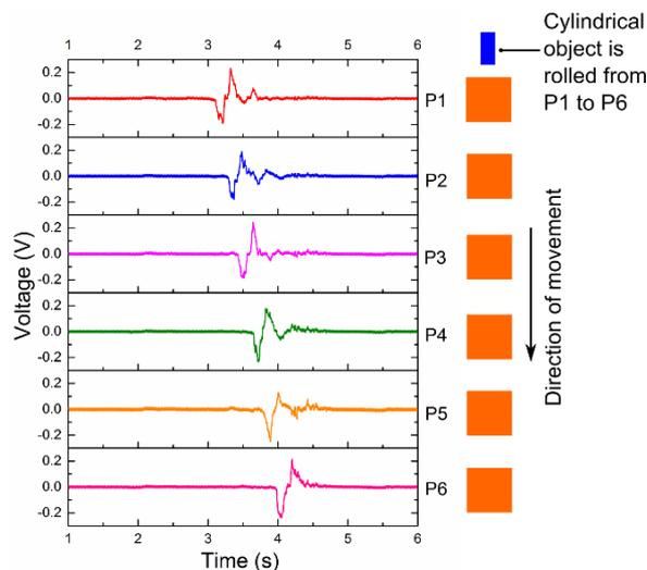
Fig. 6. Time domain output voltage signals generated by an array of 6 pixels as a cylindrical object is rolled from P1 to P6. The pixels generate a signal as the object contacts the pixel.
