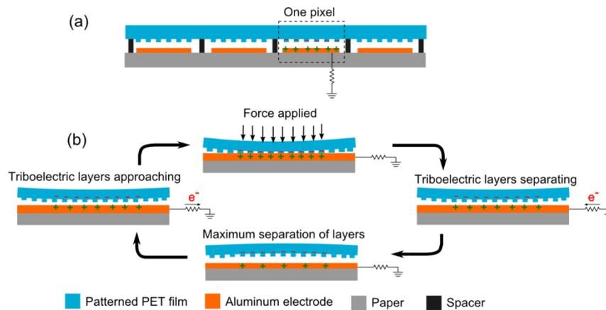
Fig. 1. (a) Schematic of pressure sensor array. (b) Working mechanism of a pixel of large scale pressure sensor array.
