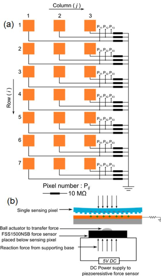
Fig. 4. (a) Schematic of pressure sensor array. (b) Setup for calibration of sensor pixels.
