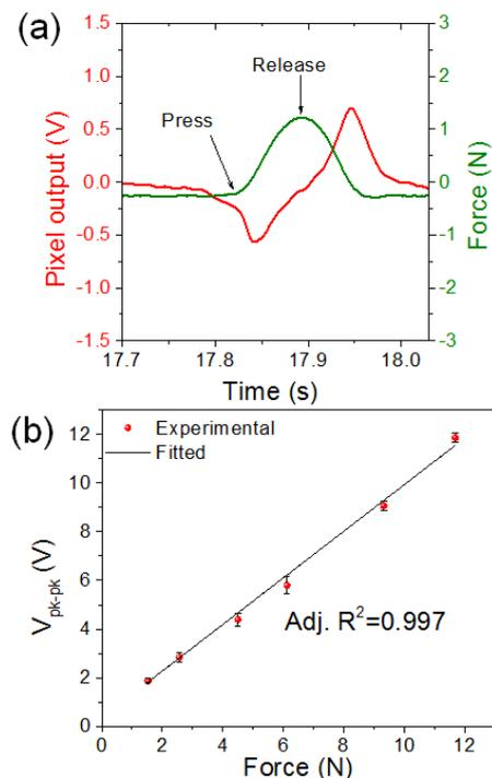
Fig. 5. (a) Time domain signal from a sensor pixel compared to a commercial force sensor. (b) Voltage output from a pixel for different value of external applied force.
