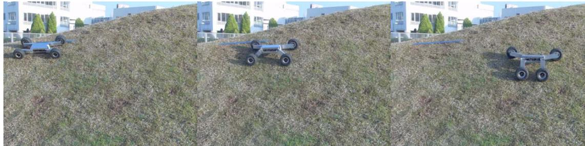
Fig. 18 Autonomous transformation control of the angle of bank by the active articulated leg and sensor
