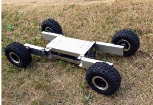
Fig. 5 The developed four wheeled reconfigurable mobile robot
