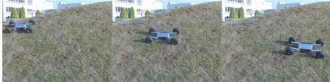
Fig. 17 An allowable sideslip of the robot in the case of  $\theta_R$  and  $\theta_L = 0$  degrees
