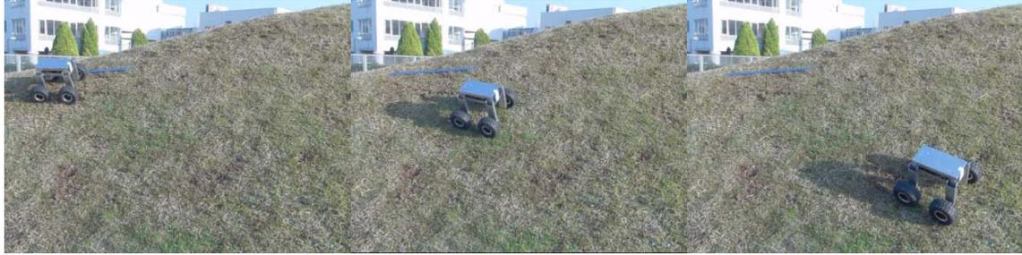
Fig. 16 An unallowable sideslip of the robot in the case of  $\theta_R$  and  $\theta_L = 90$  degrees
