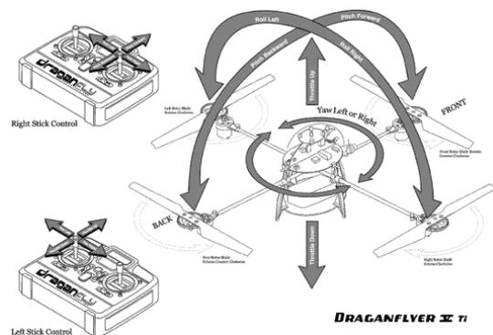
Fig. 8 The control methodology of Quadrotor
