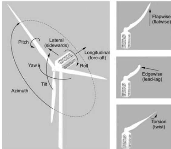
**Fig. 1** Terminology for degree-of-freedom of wind turbines [6]
