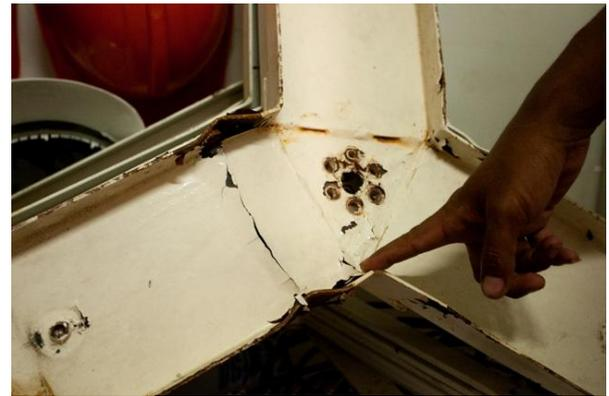
**Fig. 2** Photograph of a damaged turbine blade bracket caused by large flapwise bending moment during a horizontal gust (taken at the wind farm on Koh Larn, Chonburi in June 2009)
