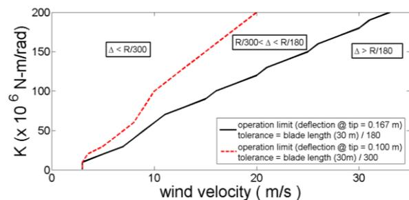
**Fig. 3.3** Diagram of bifurcation boundaries which shows regions of different values of maximum oscillation amplitudes with variation in wind velocity and flapping spring stiffness.  $\Delta$  denotes steady state oscillation amplitude.
