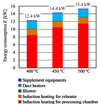
Figure 3. Electric consumption in steady state condition
