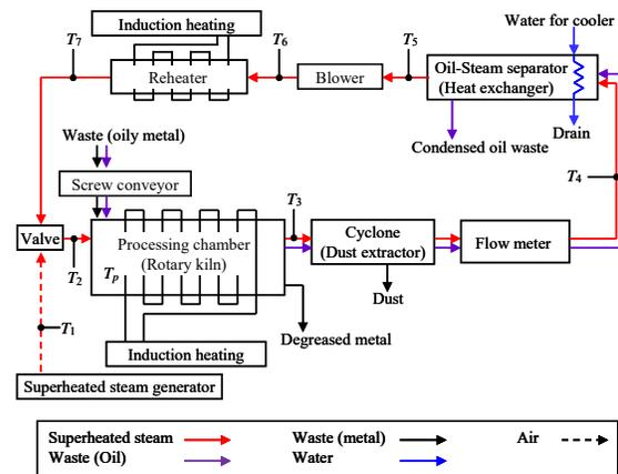
(a) System configuration of degreasing systems using superheated steam, and the position of typical local temperatures
