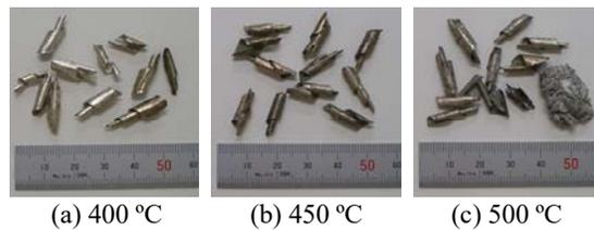
Figure 5. Degreased aluminum waste for each operation temperature
