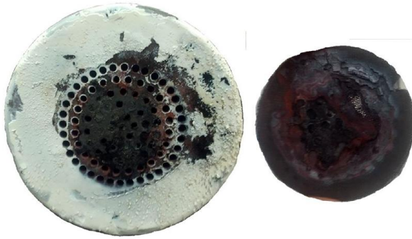
Fig. 1. The clogging of fuel outlet (left) and stainless steel wire mesh(right) [12].
