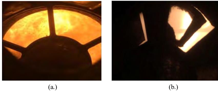
**Figure 8** the shade of flame on burner with (a.) bluff body and (b.) second swirl plate
