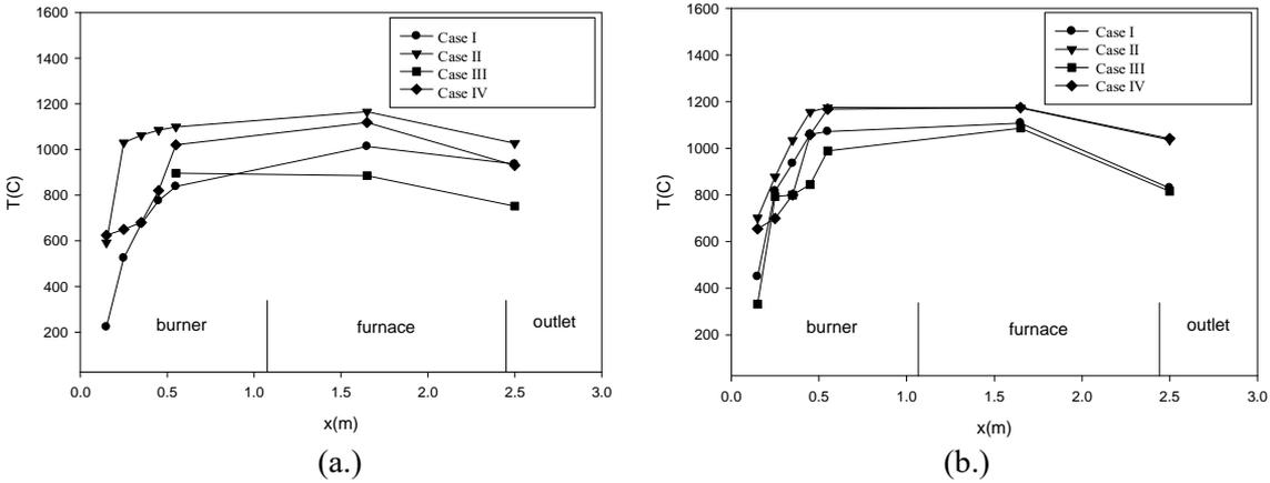
Figure 5 Axial temperature along centerline of burner from (a.) experiment and (b.) simulation
