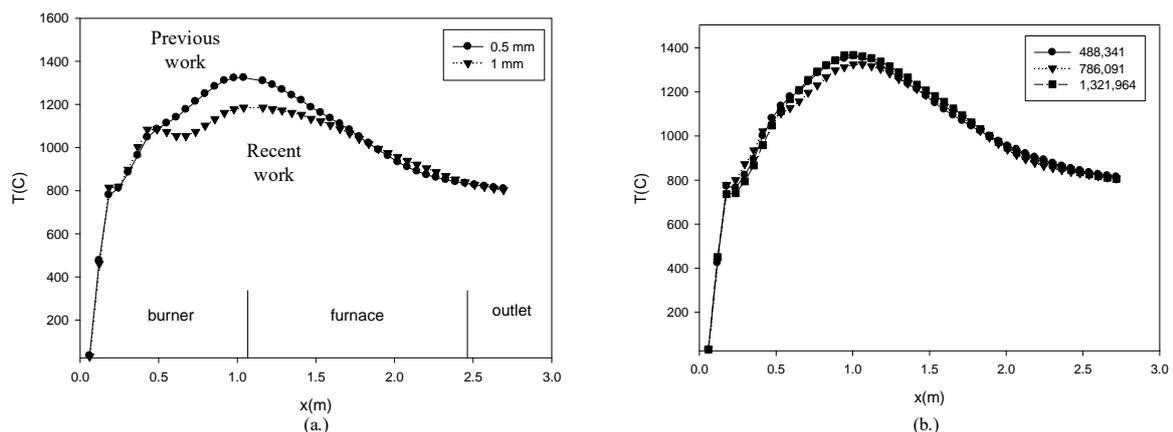
**Figure 4** (a.) Effect of particle size on axial temperature profile and (b.) Grid independence result
