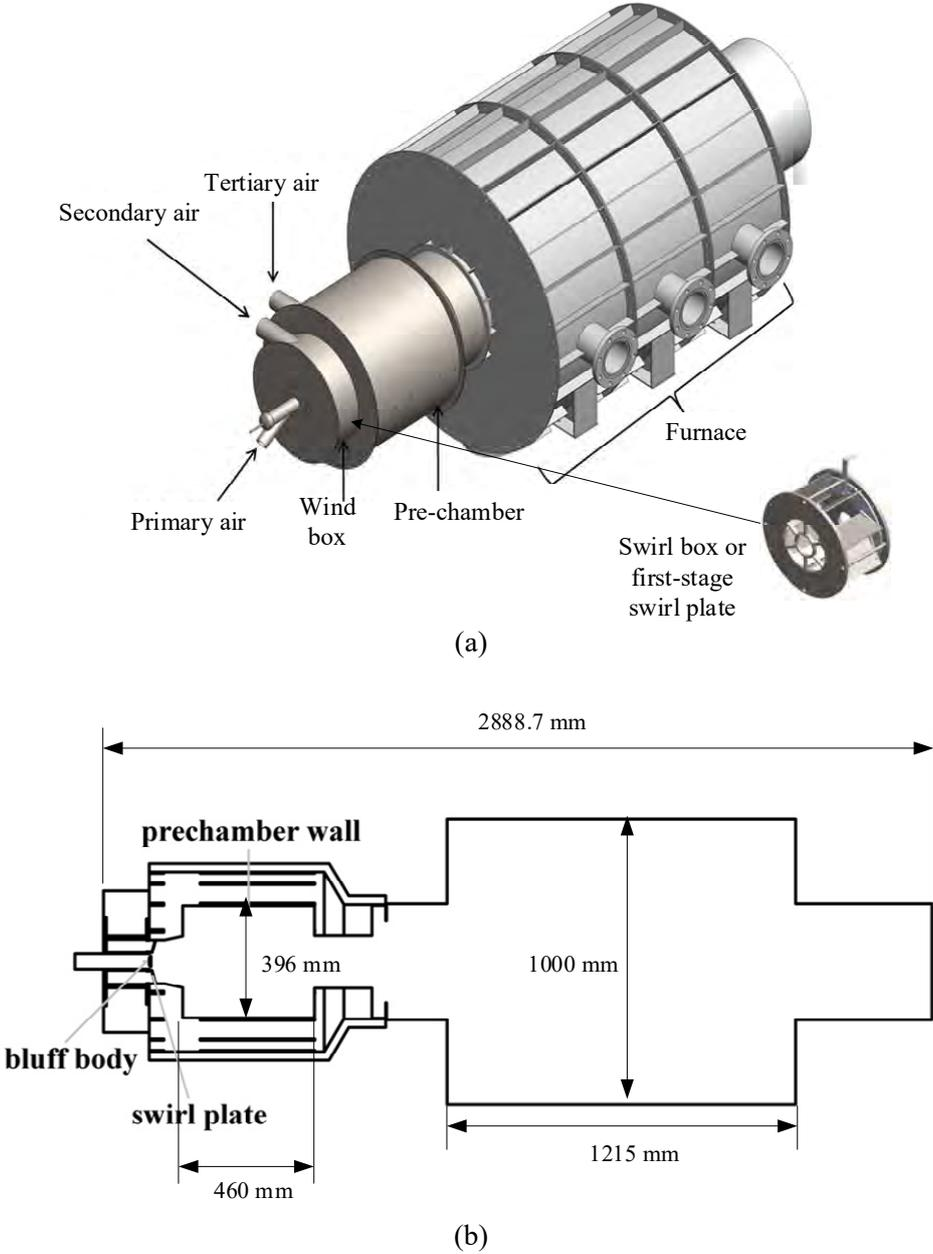
**Figure. 1** (a) Biomass burner with pre-chamber and (b) its cross section
