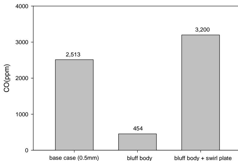
**Figure 9** CO concentration from both experiment and simulation
