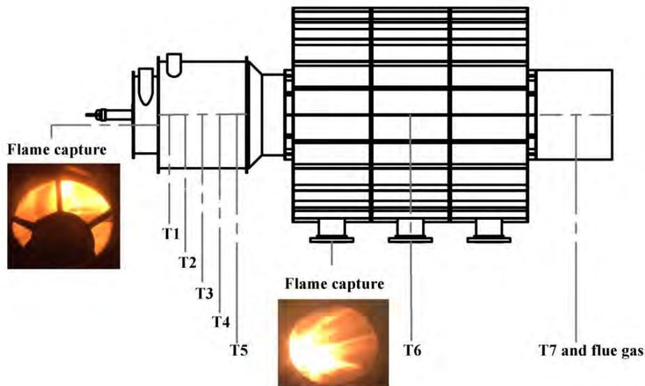
**Figure 3** Measurement and location
