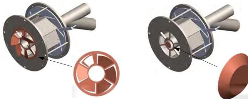
**Figure 2.** location of a.) second-swirl plate and b.) Bluff body
