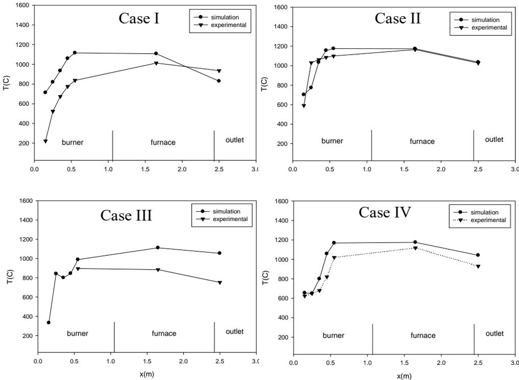
Figure 6 Comparison of Experiment and Simulation
