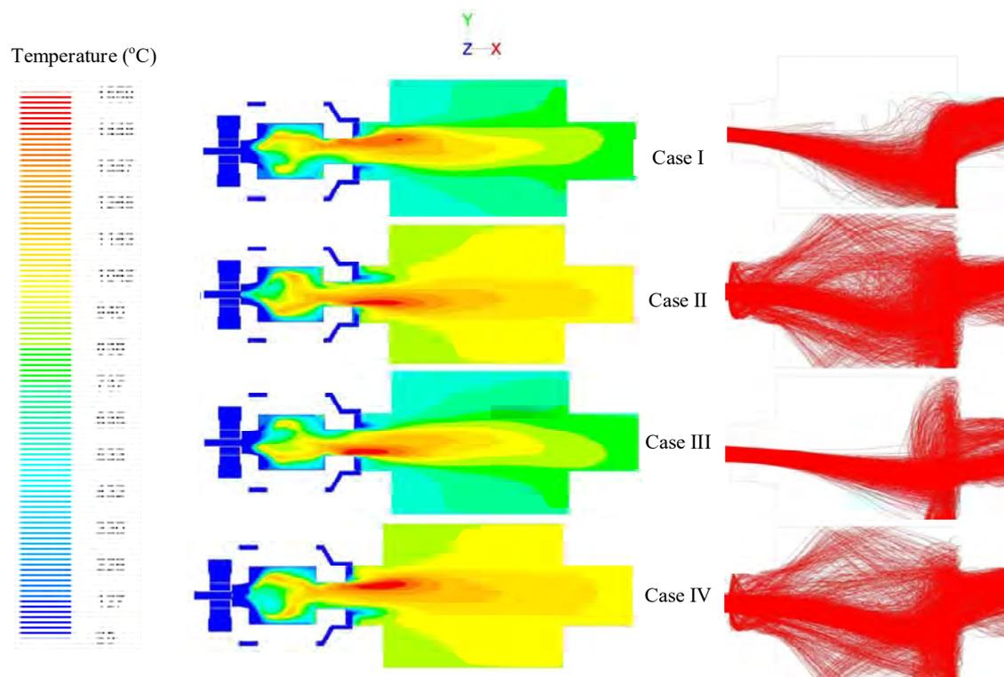
**Figure 7** Temperature Contour from simulation and Particle tracking in Pre-chamber
