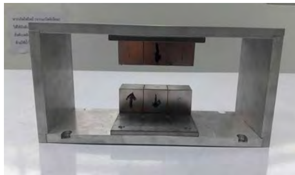
Fig.5 The magnet assembly (according to set C simulation as in Fig.3 in previous section)
