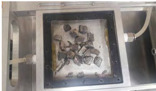
Fig.6 The regenerator with Gadolinium
