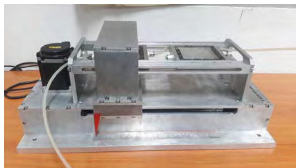
Fig.6 The regenerator with Gadolinium
