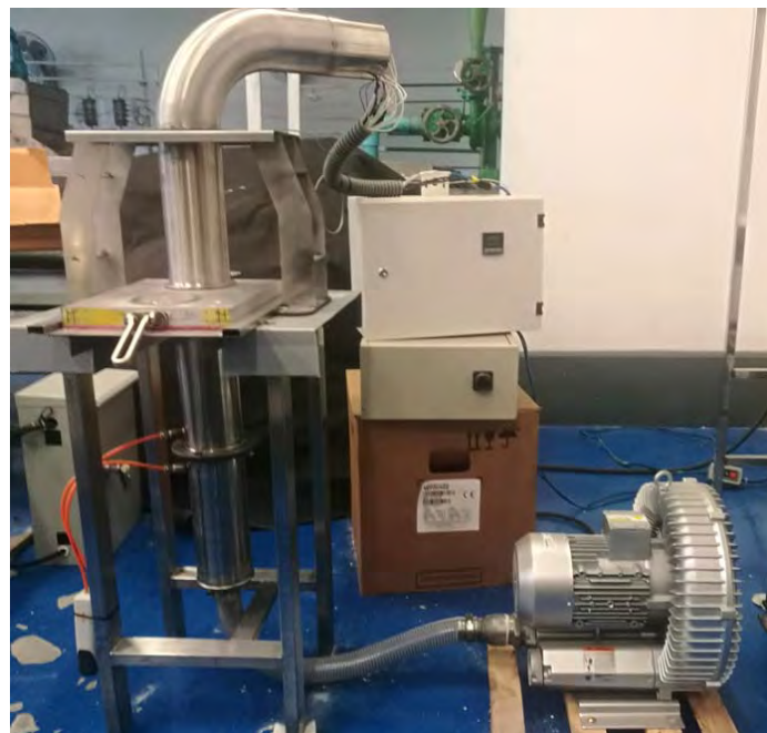
Figure 4. The air flow through dryer system.
