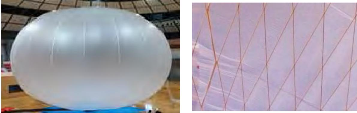
Figure 2. Super-pressure balloon(left) and balloon's surface(right)
