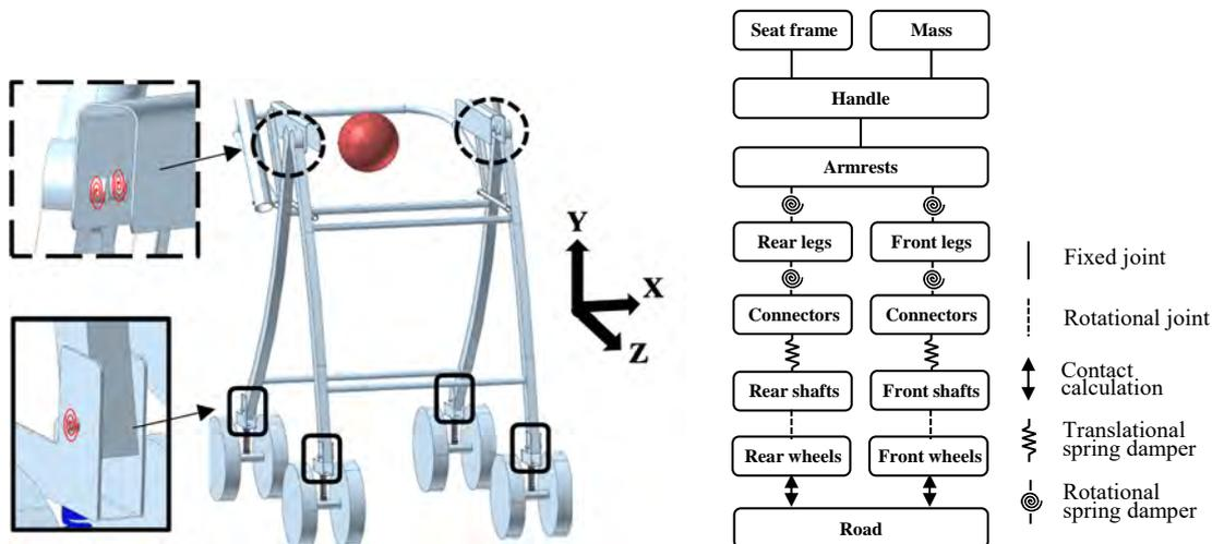
(a) Modeling points in joints of baby carriage (b) System schematic of elastic-connection model
