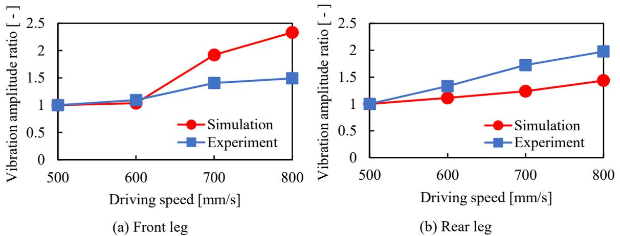
**Figure 7.** The comparison of experimental result with simulation result in influence of driving speed.
