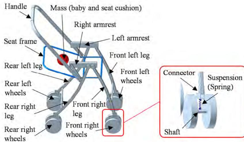
**Figure 3.** Structure of baby carriage model.
