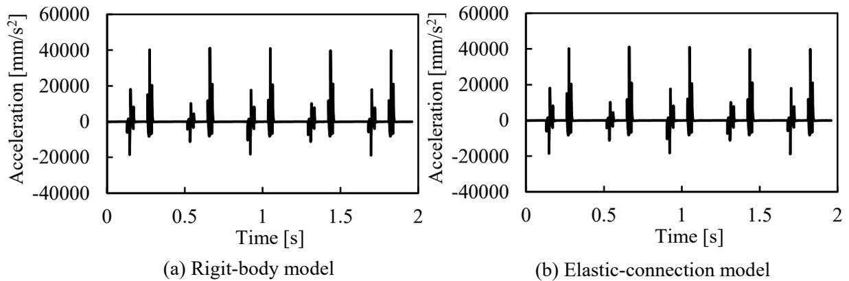
**Figure 6.** Simulation results of front leg when the driving speed is 800 mm/s.
