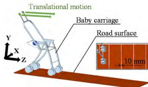
**Figure 2.** Comprehensive view of MBD simulation model.
