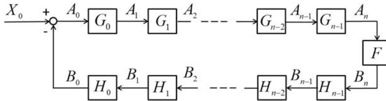
Figure 4. Block diagram of the wave control method.
