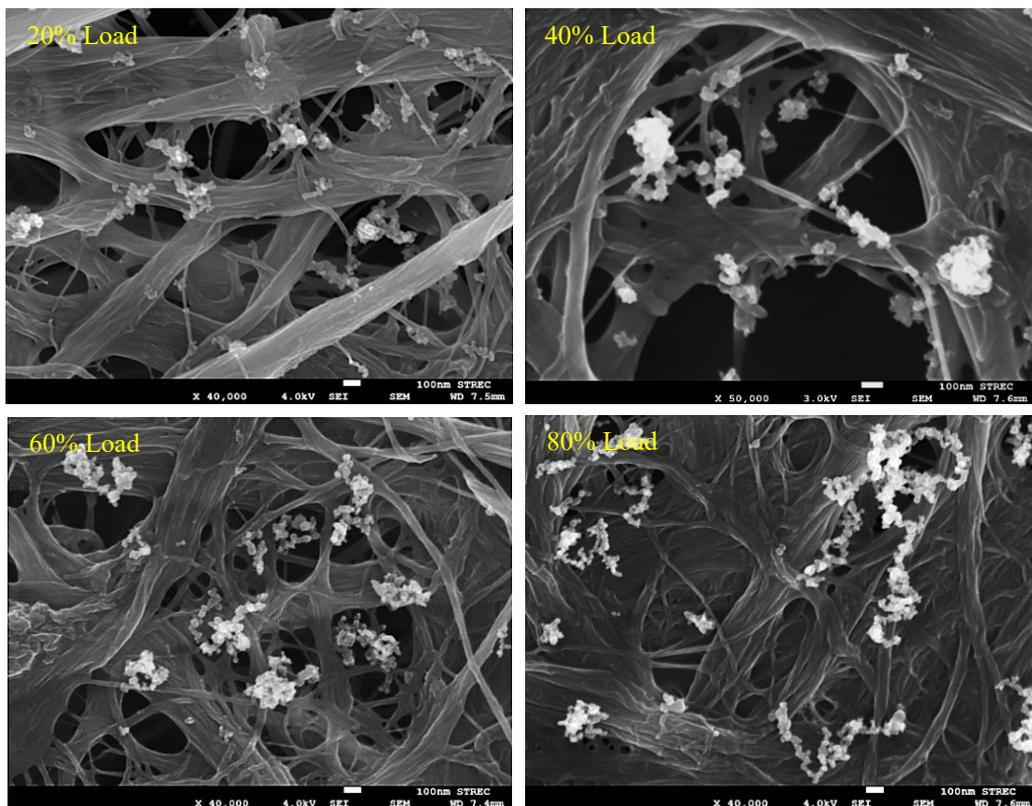
**Figure 4.** Size distribution of diesel PMs by SEM with constant engine speed 2,400 rpm.
