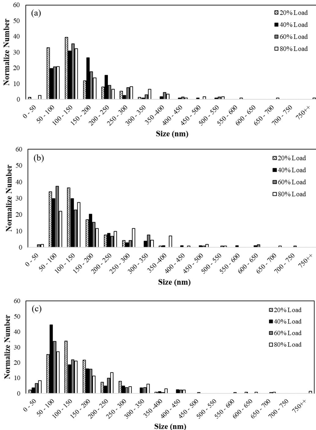
**Figure 5.** The agglomerate size distribution of diesel PMs using image processing with constant engine speed (a) 1,600 rpm (b) 2,000 rpm (c) 2,400 rpm
