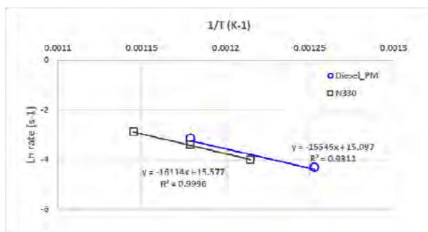
**Figure 7.** Arrhenius plots of PMs oxidation with air
