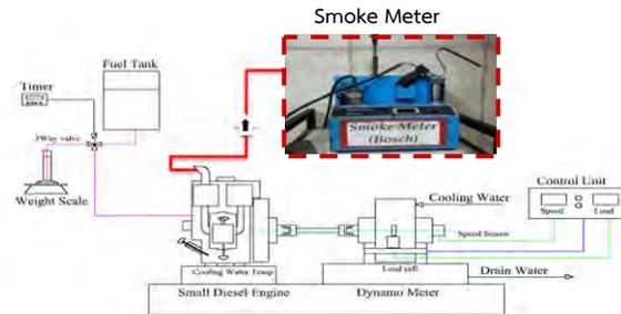
**Figure 1.** Schematic diagram of trapping particulate matter in smoke meter
