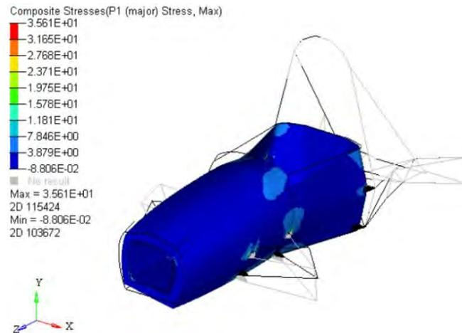
**Figure 7.** Maximum stress under couple force of  $[F_6/\text{core}/F_6]$  lay-up.
