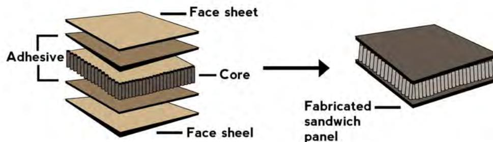
**Figure 2.** Sandwich structure with honeycomb core.
