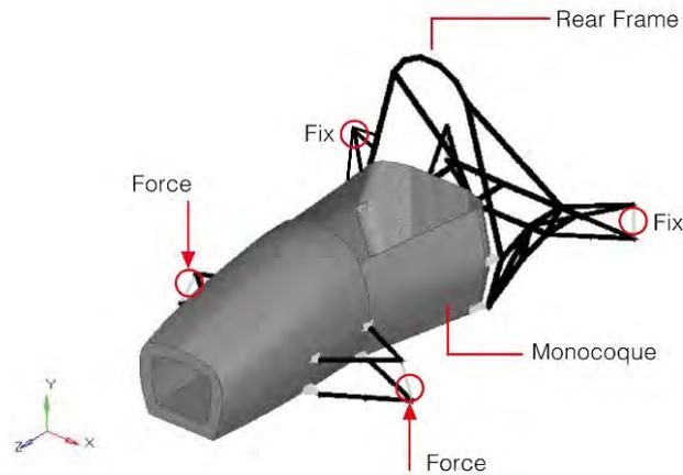
**Figure 6.** Finite element model for torsional stiffness analysis.
