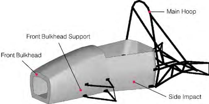
Figure 5. Monocoque structure with rear space frame.
