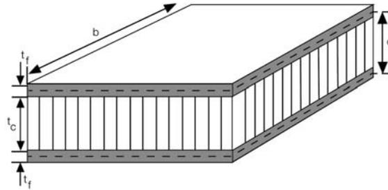
**Figure 3.** Honeycomb sandwich panel.
