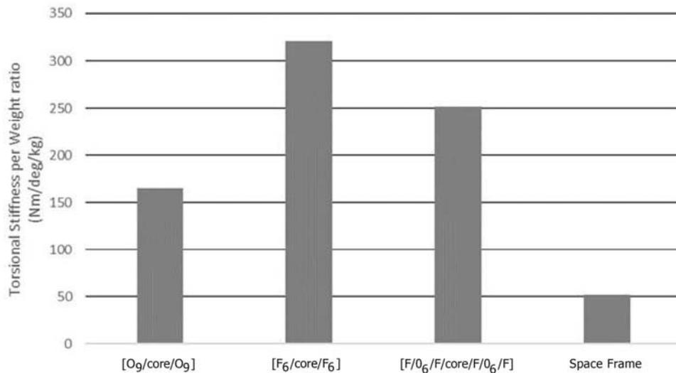
**Figure 8.** Torsional Stiffness per weight ratio comparison.
