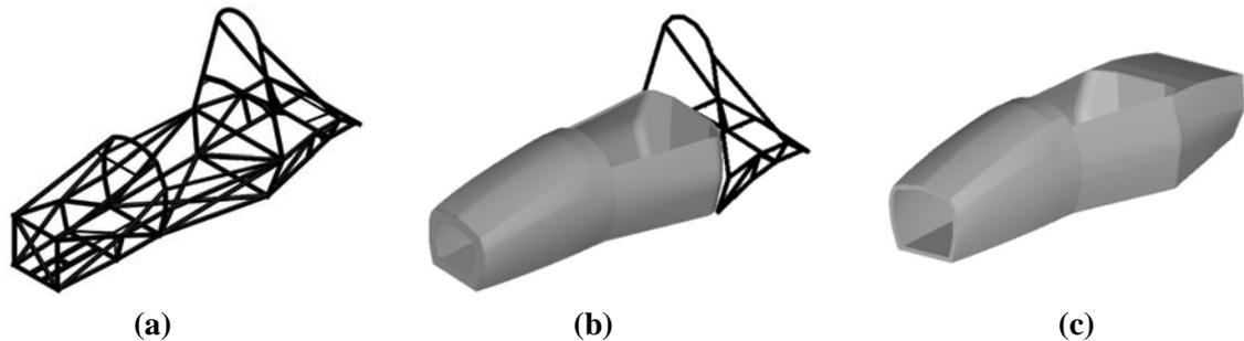
**Figure 1.** Different types of Formula Student racing car structure
