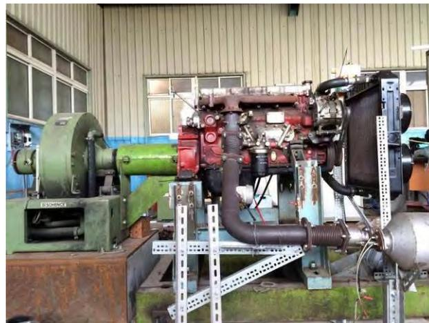
**Figure 1.** The engine and the dynamometer for the experiment
