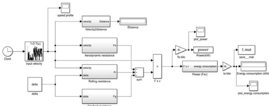
**Figure 6.** Matlab Simulink for Energy Consumption Calculation
