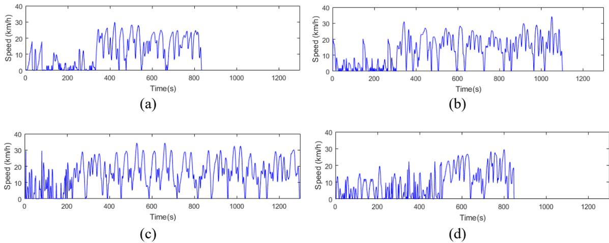
**Figure 7.** The chosen representative driving cycles for surveyed service trams (a) route 1, (b) route 2, (c) route 3, and (d) route 4
