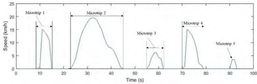
**Figure 3.** Example of microtrips segmentation from a speed-time data
