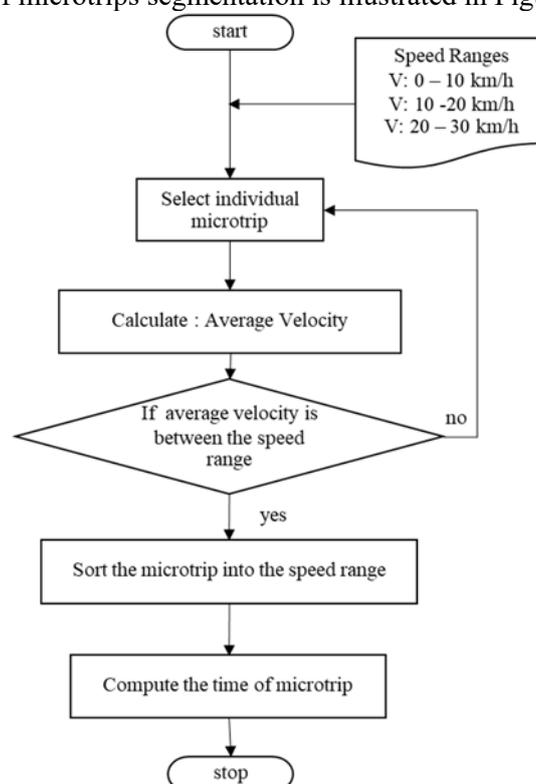
**Figure 2.** Microtrips construction process
