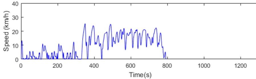
**Figure 5.** Example of tram generated driving cycle
