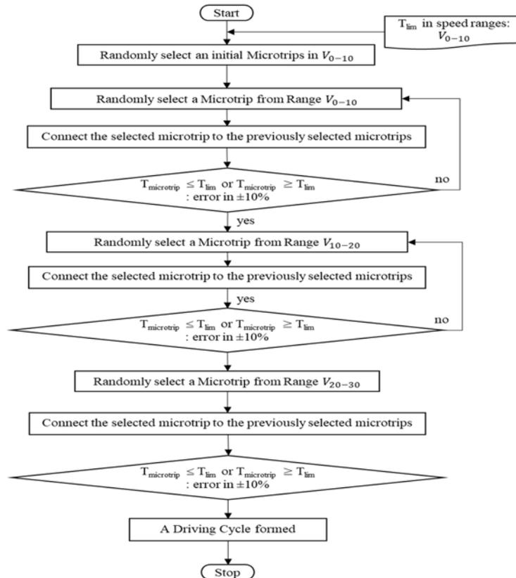
**Figure 4.** Driving Cycle Construction Procedure Flow Chart
