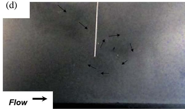
Fig. 3 Flow visualization in various  $\theta$  : (a)  $\theta = 45^\circ$  (b)  $\theta = 135^\circ$  (c)  $\theta = 225^\circ$  and (d)  $\theta = 315^\circ$
